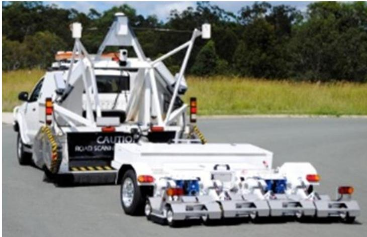
**Figure 2.8.3(c) – Example of an air-coupled antenna mounted on the front of a vehicle**
