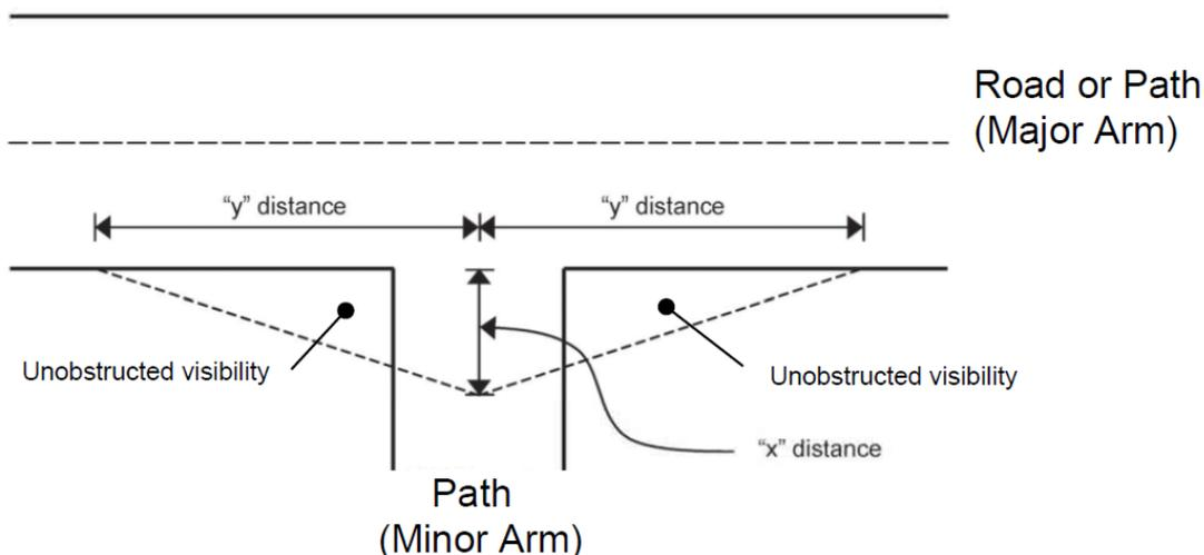
Visibility splays at intersections of paths should be provide in accordance with Figure 6A-2 where:
