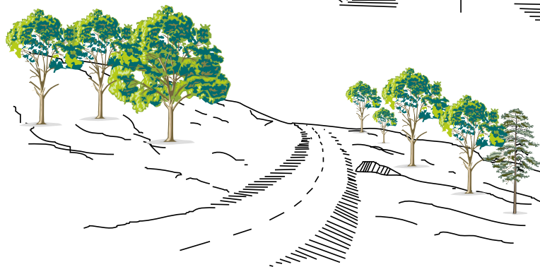
Re-aligned to fit landscape; additional excavation on road side to eliminate residual mound.
