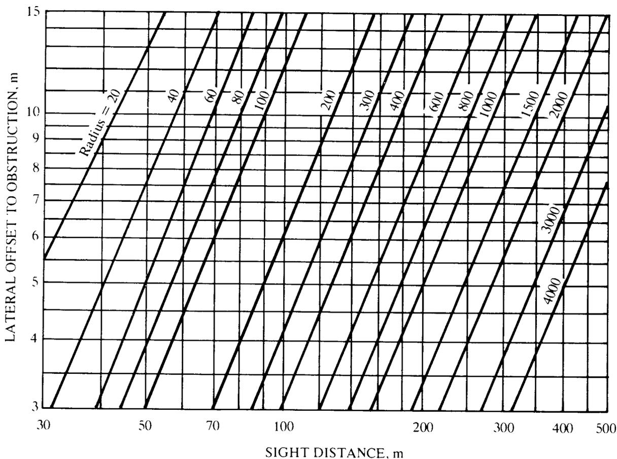
Figure 11.6 Horizontal Stopping Sight Distance for Type F Restriction to Visibility (Reaction Time = 2.5 seconds)
