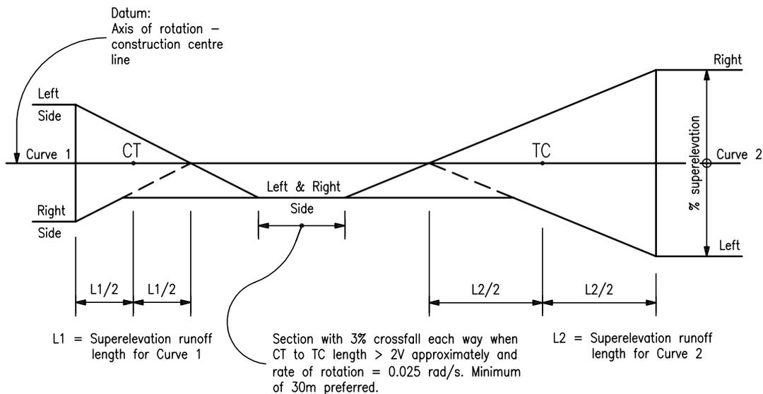
Case 5: REVERSE CIRCULAR CURVES SPACED SO THAT THERE IS A SECTION OF TANGENT WITH NORMAL CROSSFALL
