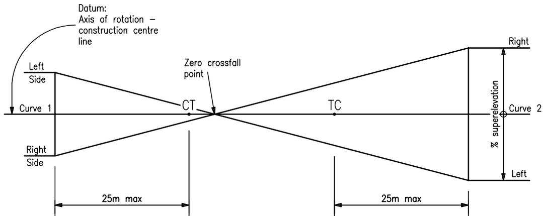
The maximum superlevation on each curve is controlled by the resultant rate of rotation of the pavement being less than the maximum for the operating speed. If this superlevation is less than that required for the curve, this case is unacceptable.
