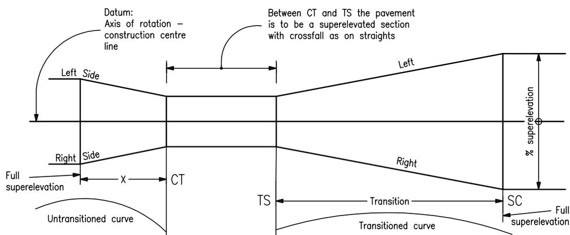
General treatment of similar curves when distance between tangent points  $< 3V$  metres ( $V$  in km/h)
