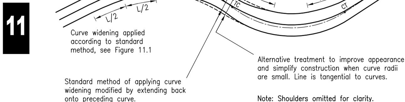
**Figure 11.5** Application of Curve Widening on Closely Spaced Reverse Untransitioned Curves
