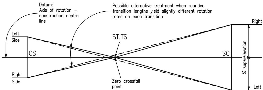
Case 1: REVERSE TRANSITIONED CURVES WITH COMMON POINT OF TANGENCY
