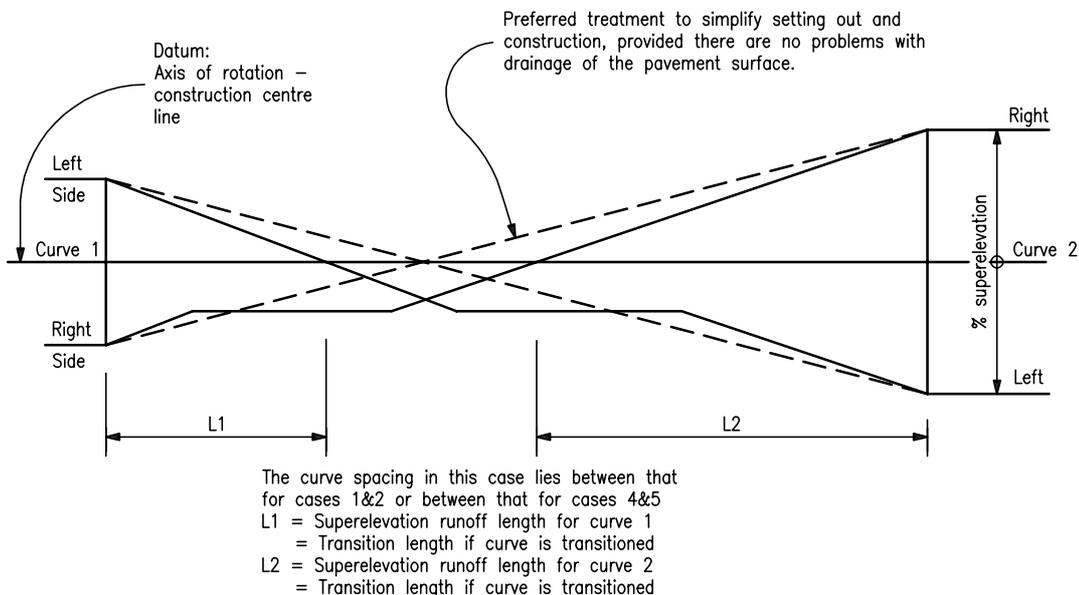
Case 6: REVERSE CURVES SPACED SO THAT THERE IS NO SECTION OF INTERVENING TANGENT WITH NORMAL CROSSFALL
