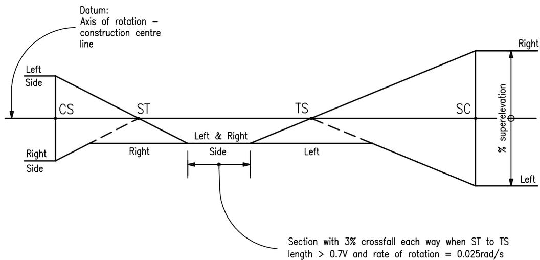
Case 2: REVERSE TRANSITIONED CURVES WITH LENGTH OF INTERVENING TANGENT > 0.7V
