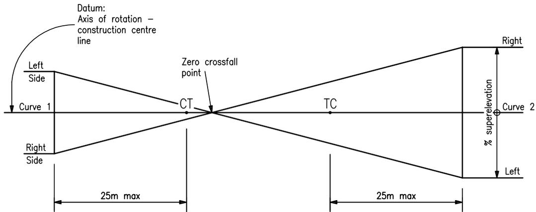
The maximum superelevation on each curve is controlled by the resultant rate of rotation of the pavement being less than the maximum for the operating speed. If this superelevation is less than that required for the curve, this case is unacceptable.
