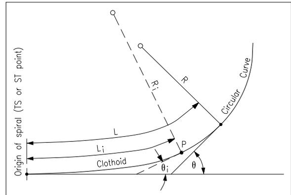
Figure 11A.1 Clothoid Spiral Transition Curve
