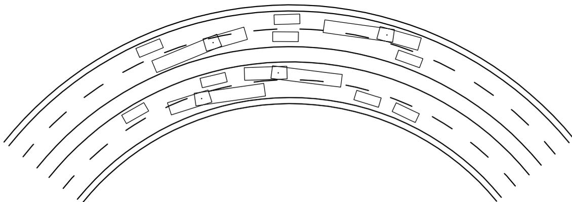
Figure 11.4 Examples of Heavy Vehicle Operation on Multi-lane Roads with Insufficient Curve Widening
