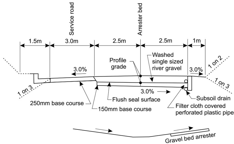
Figure 15.4 Typical Design for Gravel Arrester Bed System
