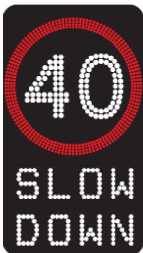
Figure 5.2© – Type 3 – School Zone Speed Limit sign Speed Activated – TC1786
