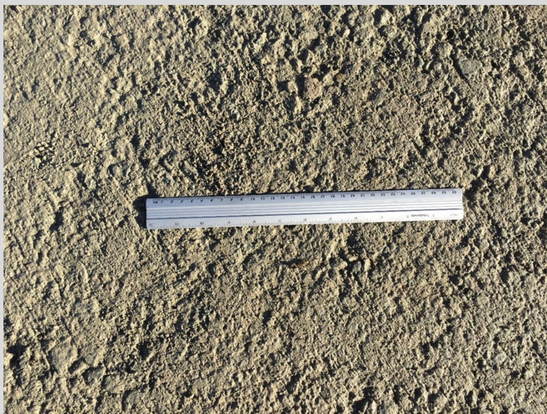
Figure 8.2.7.2 – Example of acceptable hard-cut surface
