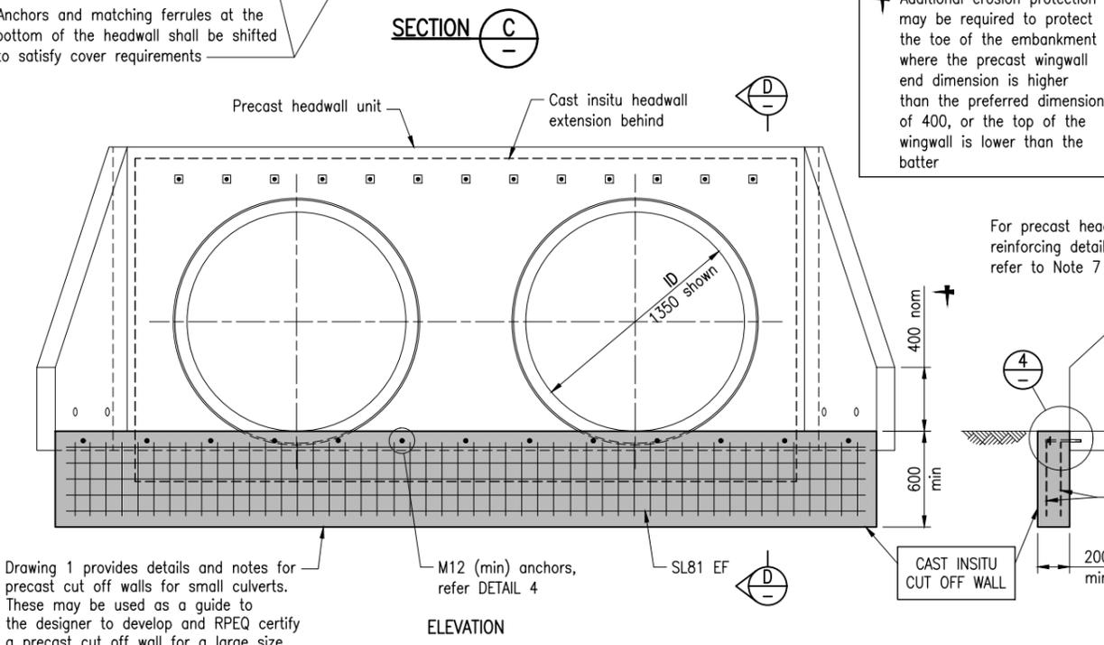
Drawing 1 provides details and notes for precast cut off walls for small culverts. These may be used as a guide to the designer to develop and RPEQ certify a precast cut off wall for a large size culvert, specific to the project
