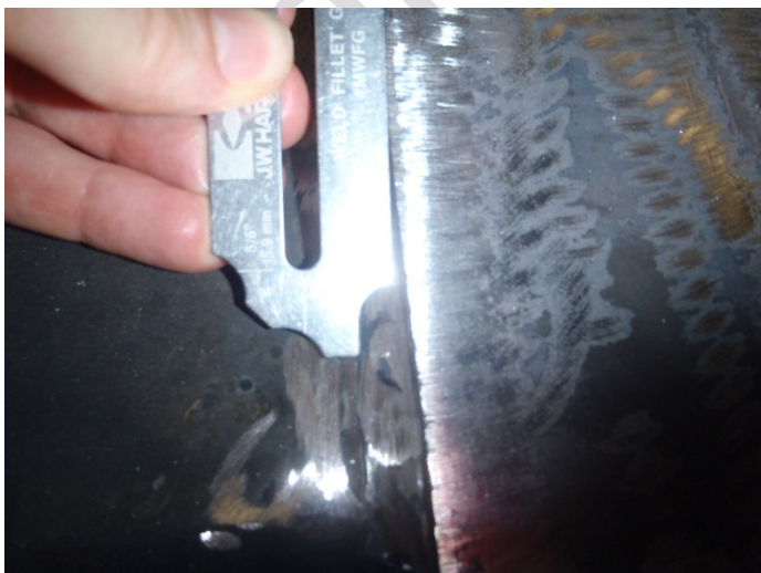
Figure 7 – Fillet weld leg length is the correct size
