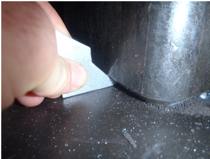
Figure 3 – View of the correct root gap between the base plate and post interface
