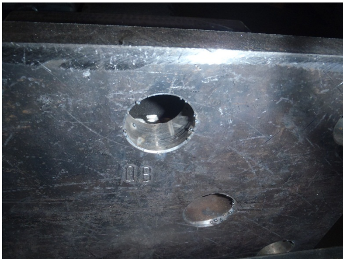
Figure 9 – View of the weld splatter in the base plate holes
