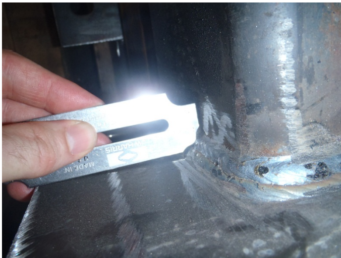
Figure 7 – Fillet weld leg length is the correct size
