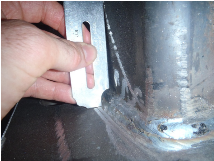
Figure 6 – Fillet weld throat thickness is the correct size
