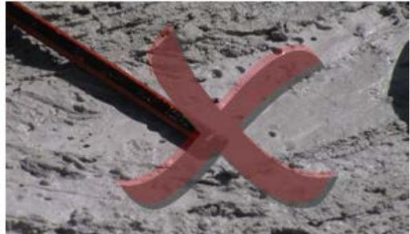
**Figure 9 Acceptable rake finish**
