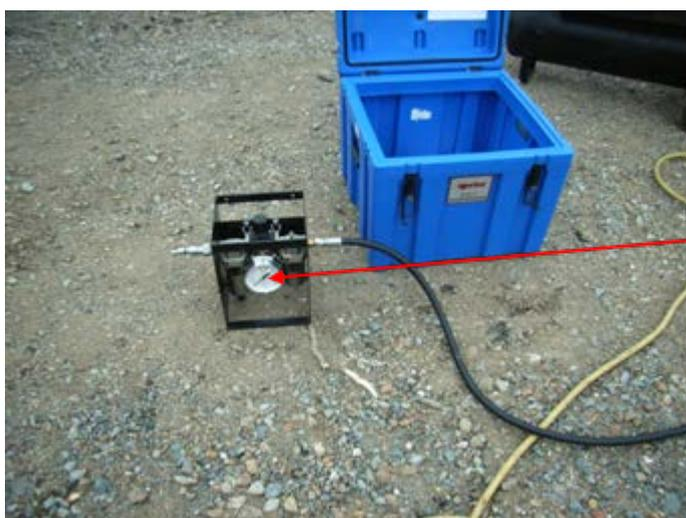
Regulator which needs to be connected to a 200cfm air compressor
