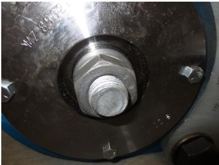
**Figure 8.2(c) – View of the bolt head in the skidmore**
