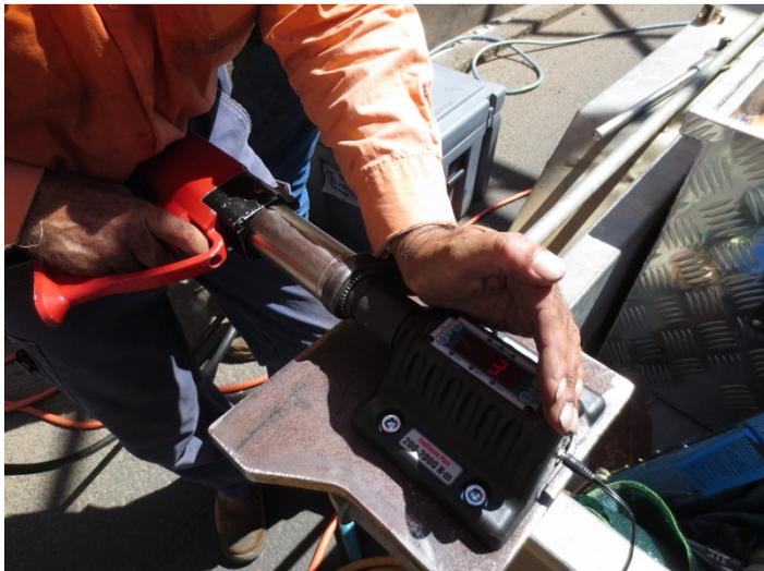
True Checker device is used to outline the torque setting for a torque wrench. Many wenchers are set via pressure and the true checker determines the torque in the torque wrench for a specific pressure. True Checker can also be used to ensure the torque in the torque wrench correctly calibrated.
