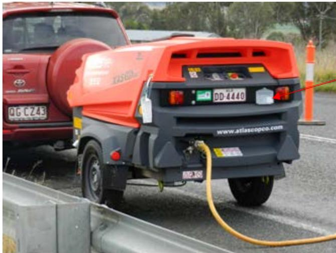
Compressor required to run the pneumatic torque wrench
