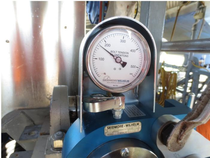
**Figure 8.2(e) – View of the torque wrench on the True Checker**
