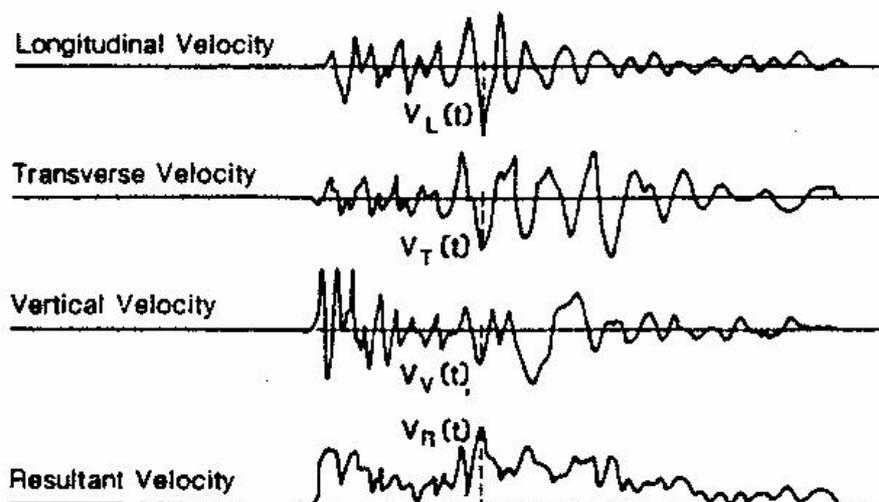
The resultant particle velocity at a given instant can be obtained by the vector sum from three mutually perpendicular geophones, i.e. resultant particle velocity at a given time (t):
