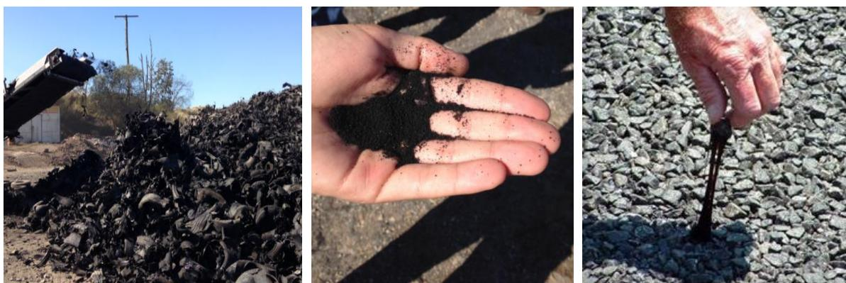
CRM binder is used extensively in sprayed sealing, with [MRTS11 Sprayed Bituminous Surfacing \(Excluding Emulsion\)](#) being updated to permit Contractors to substitute a CRM binder in many cases where a conventional polymer modified binder (PMB) is specified. CRM sealing binders can be either field or factory blended products and usually contain approximately 15% crumb rubber.
