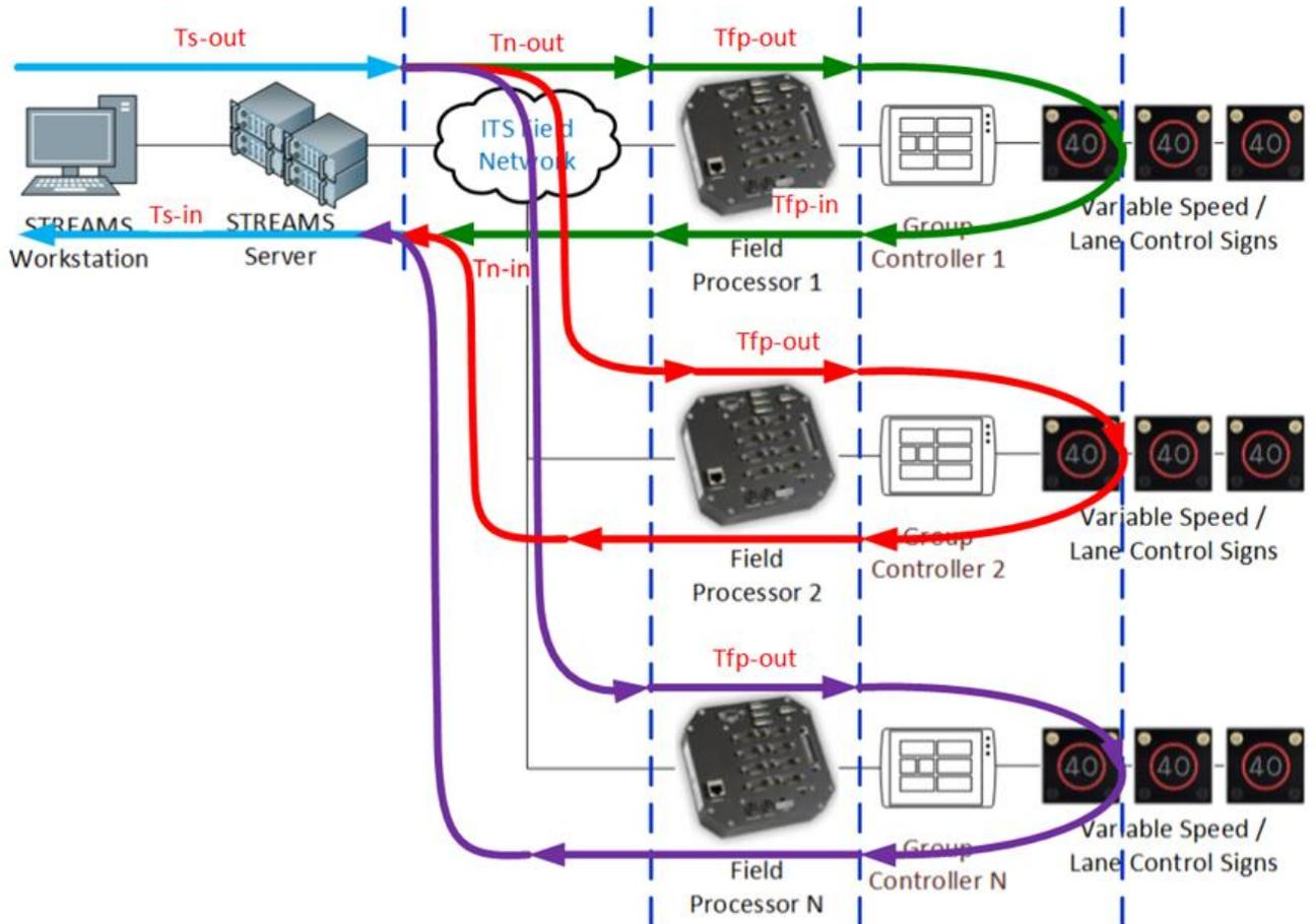
The diagram above can also be represented as a timing diagram shown in Figure 4-B. The arrows in the diagram show the movement of information required to implement a LUMS Response Frame across a set of gantries.
