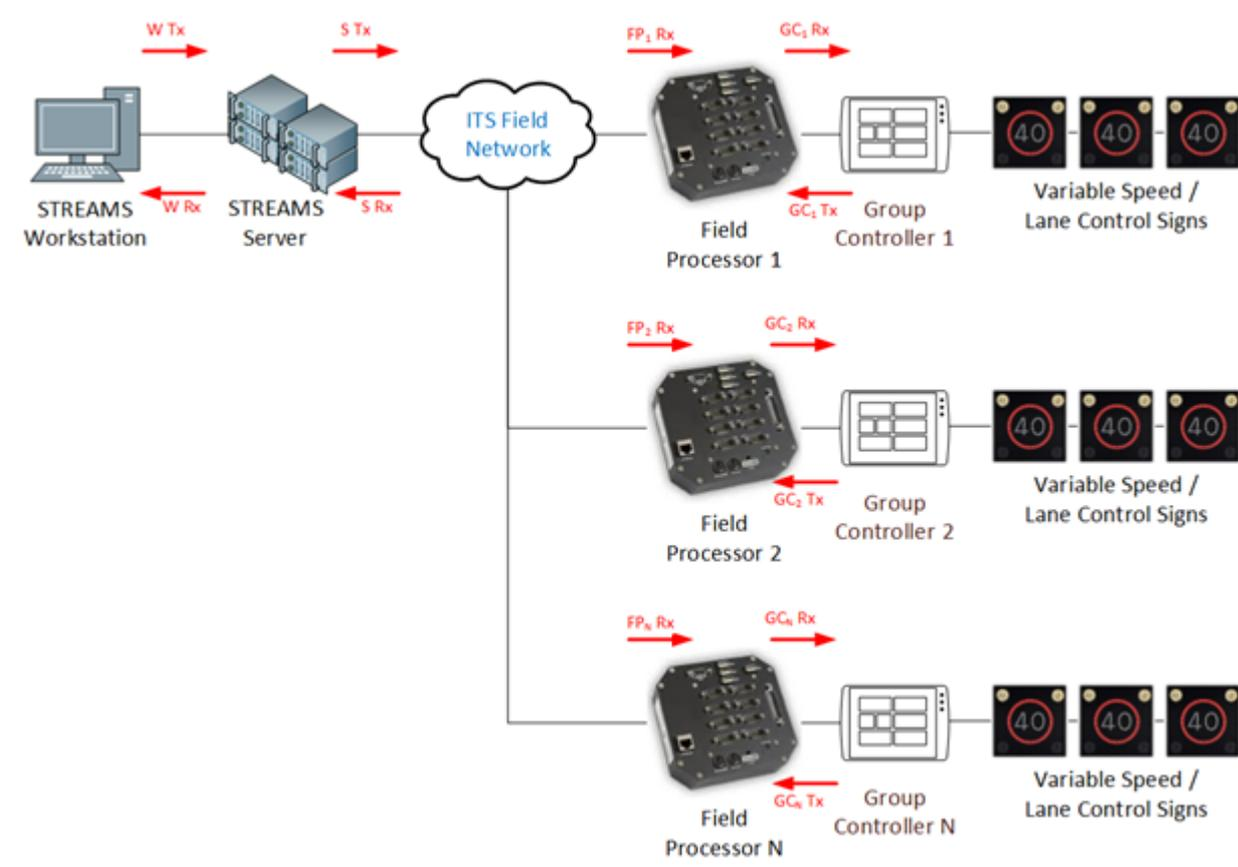
In the above diagrams, the red arrows indicate the messages that are transmitted and/or received by each device. The following descriptions apply:
