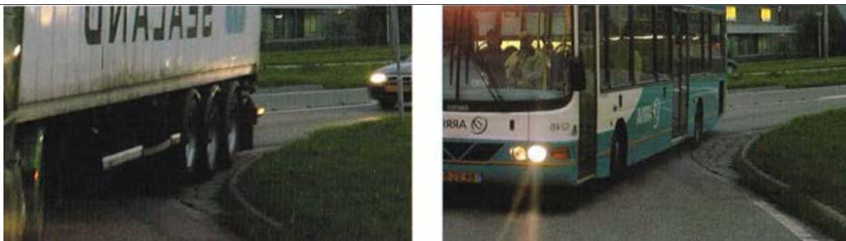
Outside Aprons. Note cobbles not preferred due to maintenance, durability and constructability Source: CROW Guide to Turbo Roundabouts 38
