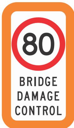
The BRIDGE DAMAGE CONTROL sign shall be mounted below the Speed Restriction sign when it is used to impose a temporary speed limit on a bridge to manage structural deficiencies.
