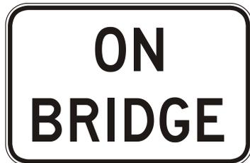
The ON BRIDGE sign shall be mounted below the Speed Restriction sign when it is used to impose a permanent speed limit on a bridge.
