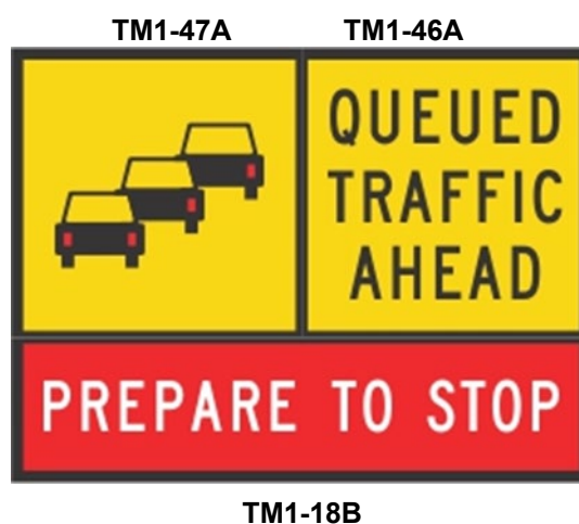
Figure 4.8(a) – Queued traffic ahead multi-message sign assembly
