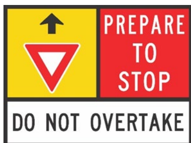
Figure 5.4.4(b) – Advance PREPARE TO STOP sign for Give Way control
