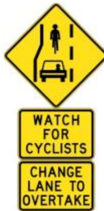
Figure 2.3(H) – TC2003 sign assembly for road or lane narrowing
