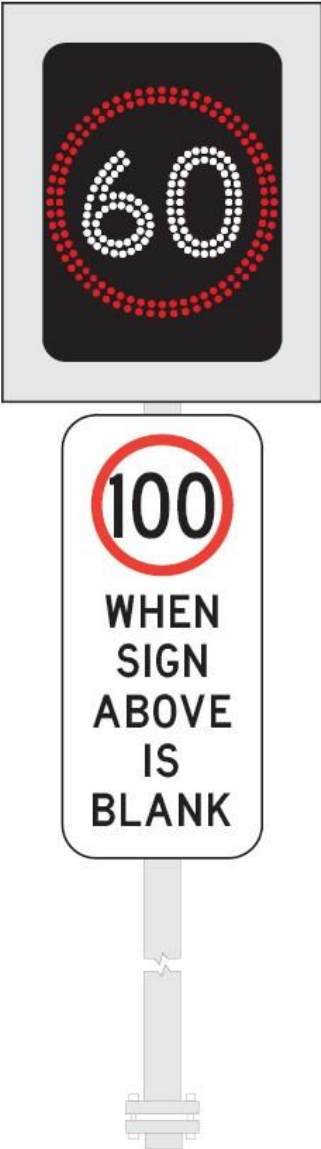
Figure 8.1 – Concept drawing for pole-mounted variable speed limit sign with supplementary static default sign (where applicable)
