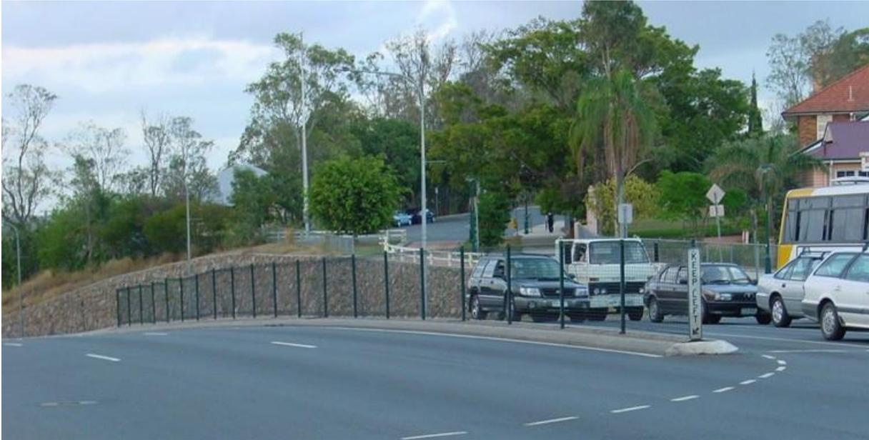
**Figure 1.1-B – When used at staged crossings on pedestrian refuges, fences should be aligned so that pedestrians face oncoming traffic as they are about to leave the median**
