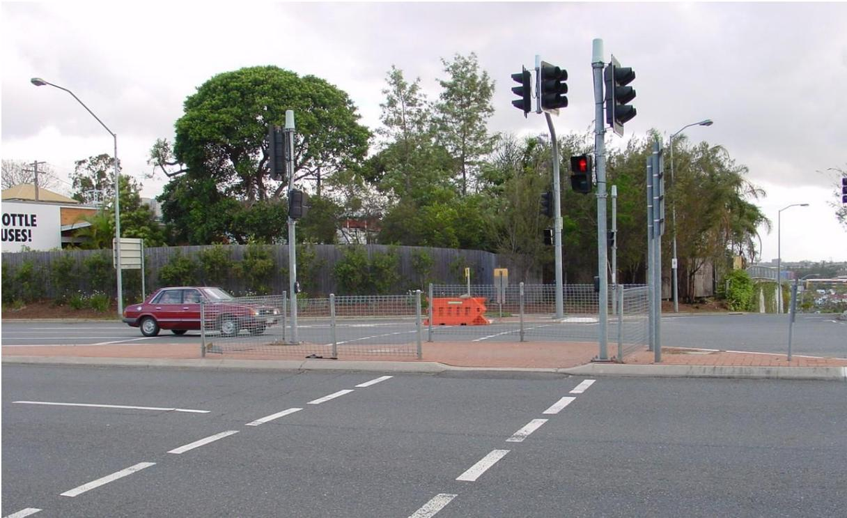
**Figure 1.1-C – Fencing and barriers constructed using a horizontal rail should not be used because of the risk of spearing pedestrians and vehicle occupants during a crash**
