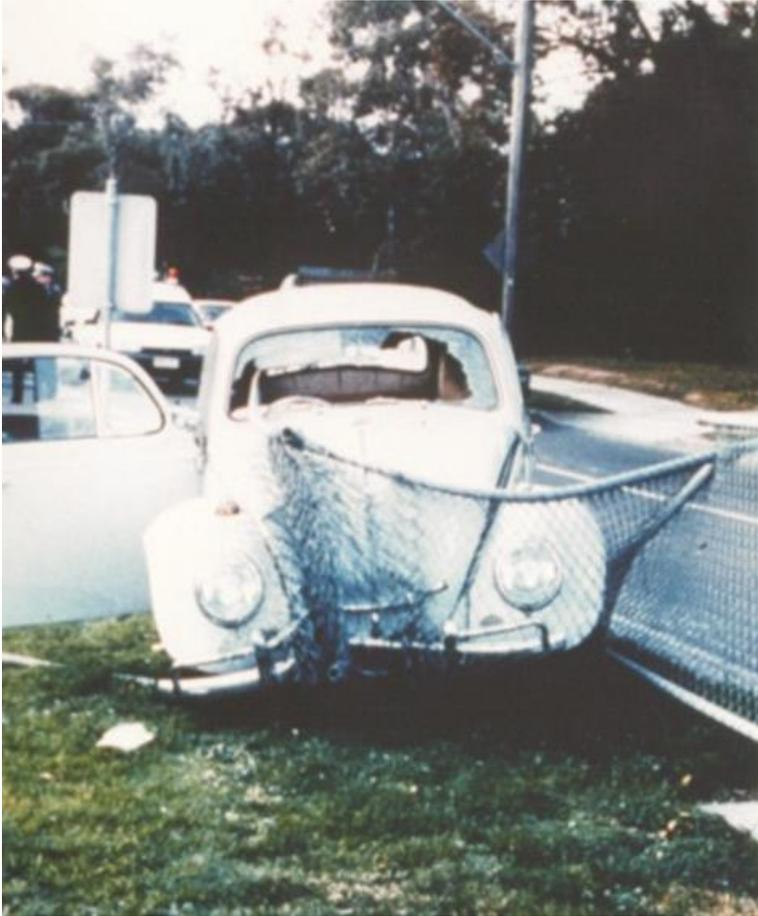
**Figure 1.1-D – Fencing and barriers constructed using a horizontal rail should not be used because of the risk of spearing pedestrians and vehicle occupants during a crash**
