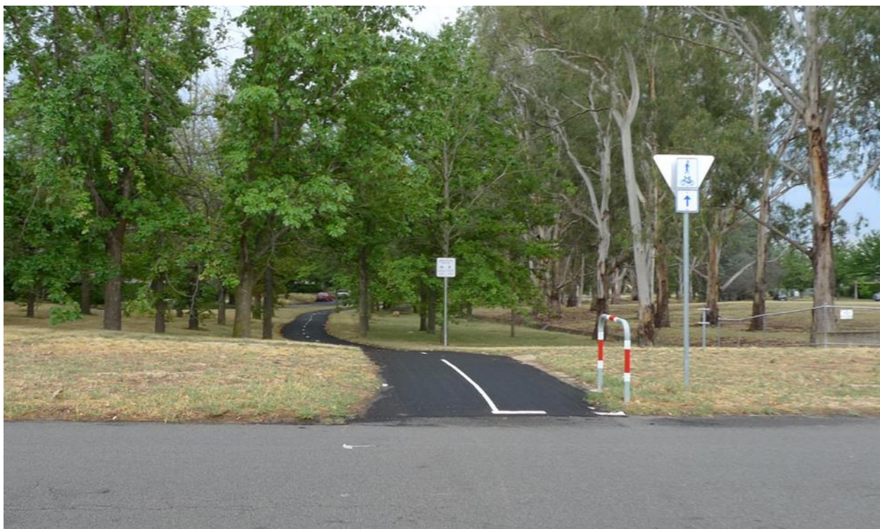
Figure 8.2.2-1 – Path with minimal termination treatment
