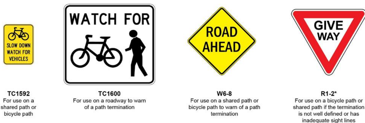
Figure 8.2.2-1.2.1 – Signs used for slowing cyclists and warning of a path termination
