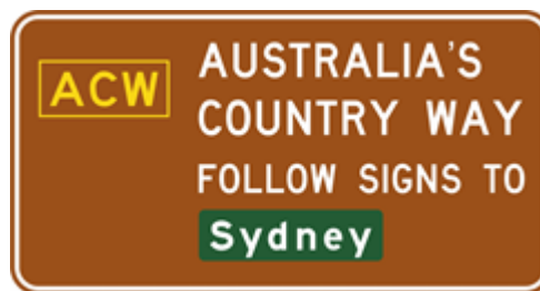
Figure 4.2(b) – Advance direction signs (TC2268)
