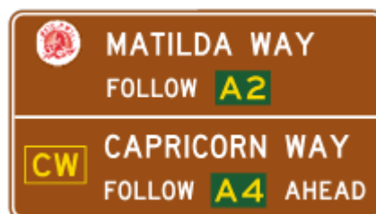
Figure 4.2(c) – Advance direction signs (TC2025)
