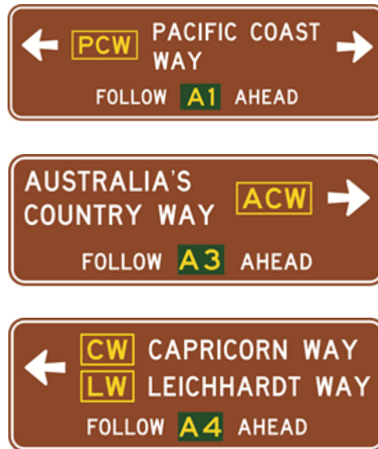
Figure 4.2(d) – Advance direction signs (TC2026)
