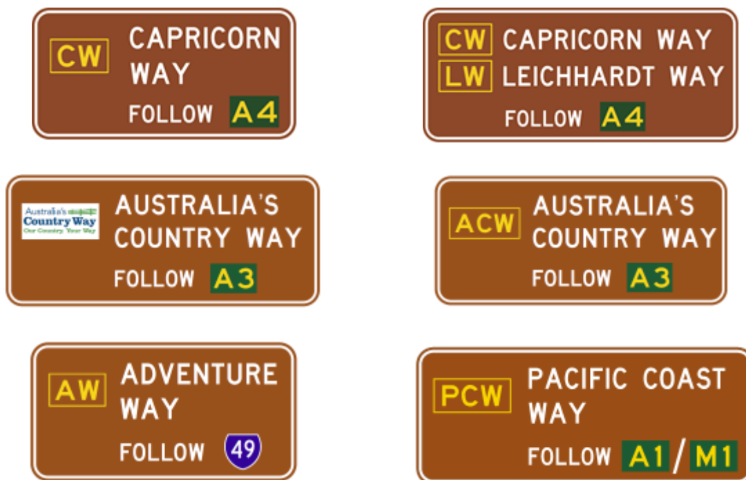
Figure 4.2(a) – Advance direction signs (TC2025)
