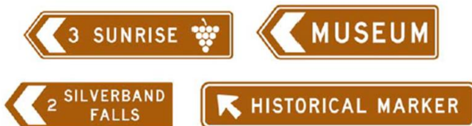
Figure 5.2.2.2 – Examples of intersection signs
