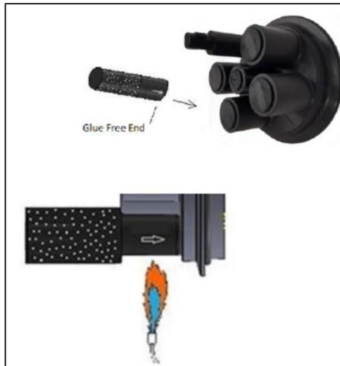
**SLEEVE** – Slide the glue-free end of the heat-shrink sleeve onto the prepared port.
