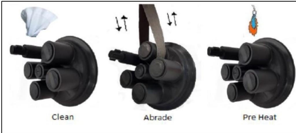
**CLEAN** – Knock out enclosure ports as required and wipe ports with a clean cloth.
