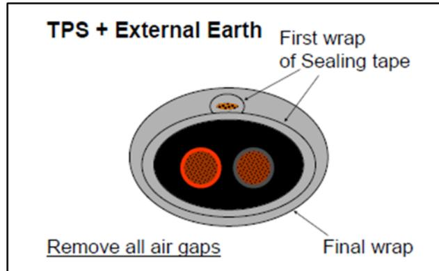
**PLACE CABLES** – Place the sealed sections of the earth and power cables together and press.
