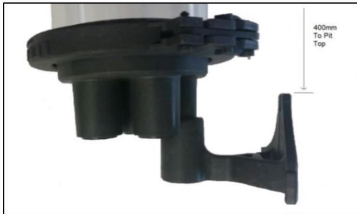
**INSTALL BRACKET** – Install joint enclosure support bracket on the inside wall of the pit at a height to allow clearance from pit lid (recommended 400 mm from top of pit to top of bracket).
