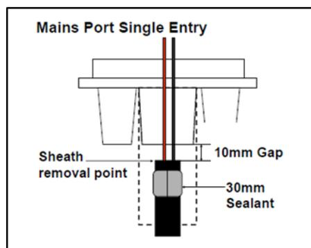
**APPLY TAPE** – Apply sealant tape to outer insulation.
