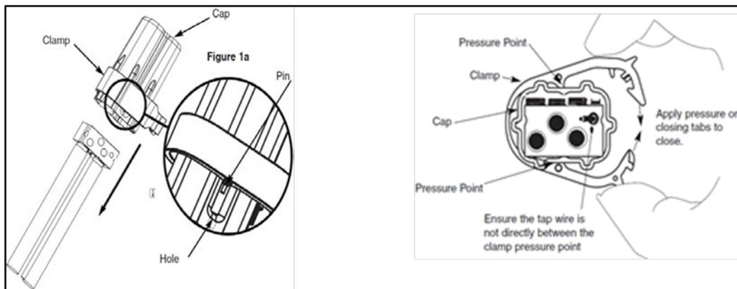
**INSTALL CAP** – Install cap by holding all wires and pushing the cap over the connection assembly until it goes no further.
