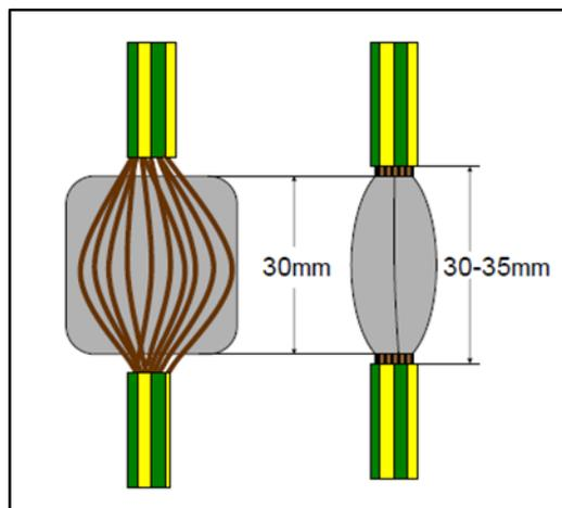
**REMOVE INSULATION** – 400 mm from the end of the cable, remove a 40 mm of green / yellow insulation exposing a 30–35 mm section of copper strands.
