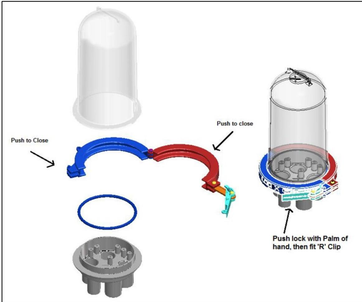
**SEALANT SET** – After the sealant is set, the joint can be closed.
