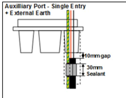
**COMBINE CABLES** – The external earth cable must be installed along with a TPS cable.
