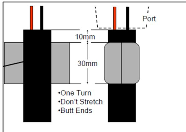
**CUT TAPE** – Cut the sealant tape to fit one turn around cable.
