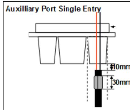
**APPLY TAPE** – Apply sealing tape to outer sheath.
