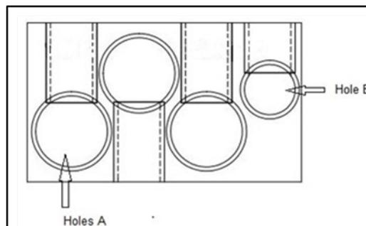
**SELECT HOLE** – Select hole in connector to suit cable size.
