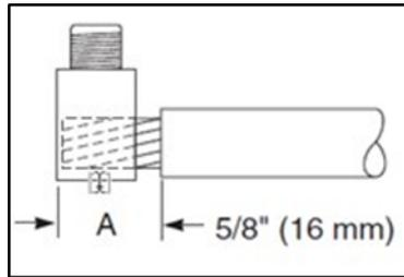
**REMOVE INSULATION** – Insulation removal length equals connector insertion depth (16 mm), allowing gap between insulation and connector.
