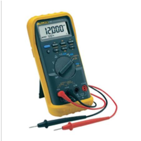
A dual impedance digital multimeter is recommended to confirm if any inducted voltages are present in high impedance CCTS that are de energised.
