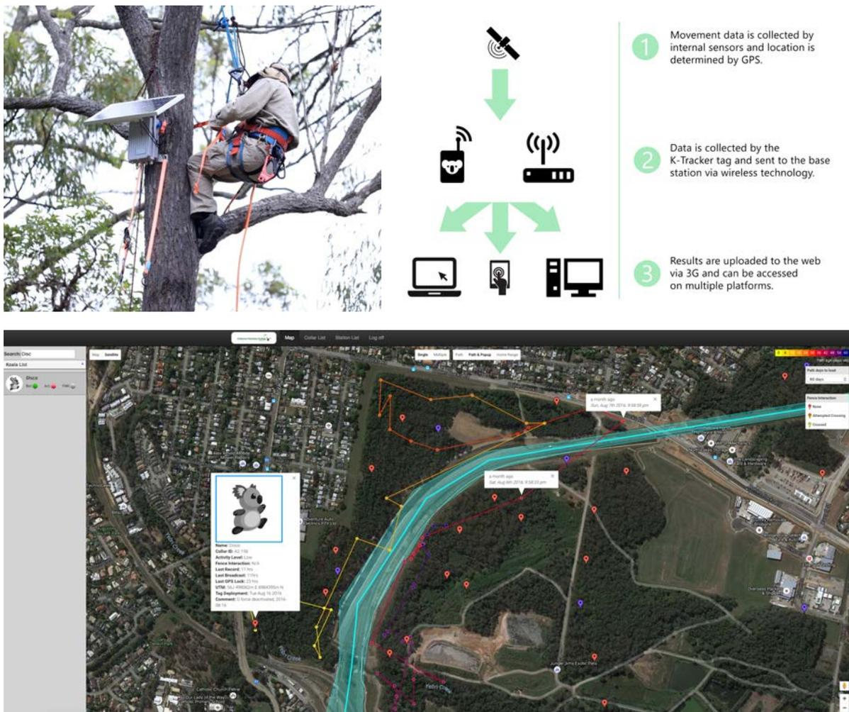
**Figure 2.5:** Data outputs from the K-Tracker collars are relayed to the LX Solutions-hosted website via solar-powered base stations. Data are displayed graphically on a Google-Earth map overlay on the website (bottom image), and are downloadable as CSV files for more detailed data processing and analysis. Top left plate shows installation of a base station at the Kippa-Ring bushland. Top right figure shows a graphical representation of the K-Tracker communications system.
