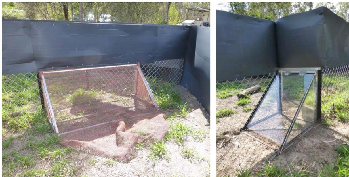
**Plate 6.6:** Two early prototypes of the koala egress valve. The left image shows a netting valve; the right image shows a horizontally-hinged Perspex® door. Both were used by trial koalas, but not consistently.
