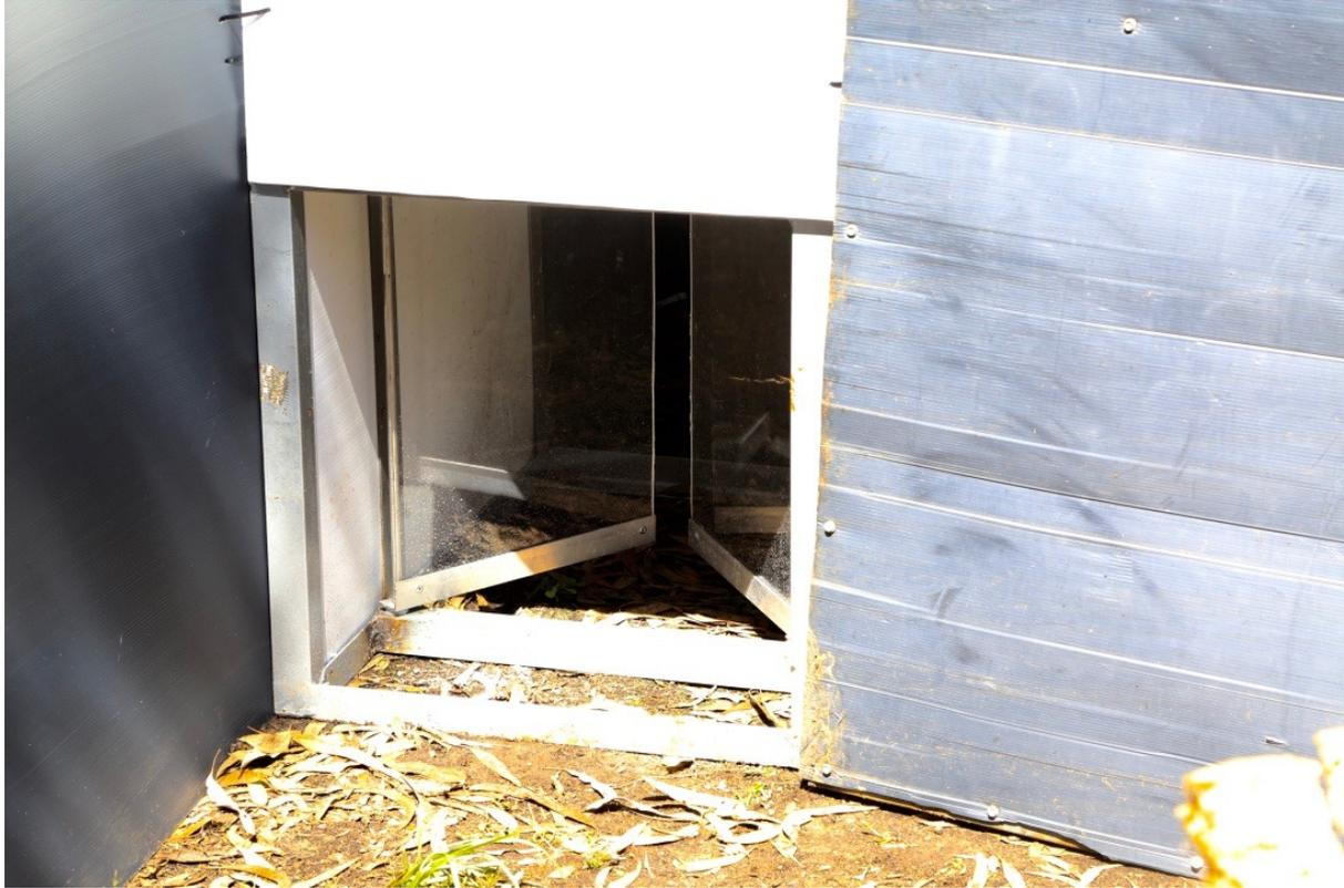
**Plate 6.7:** Prototype of the most successful koala egress valve, with two vertically-hinged, lightly-sprung Perspex® doors.
