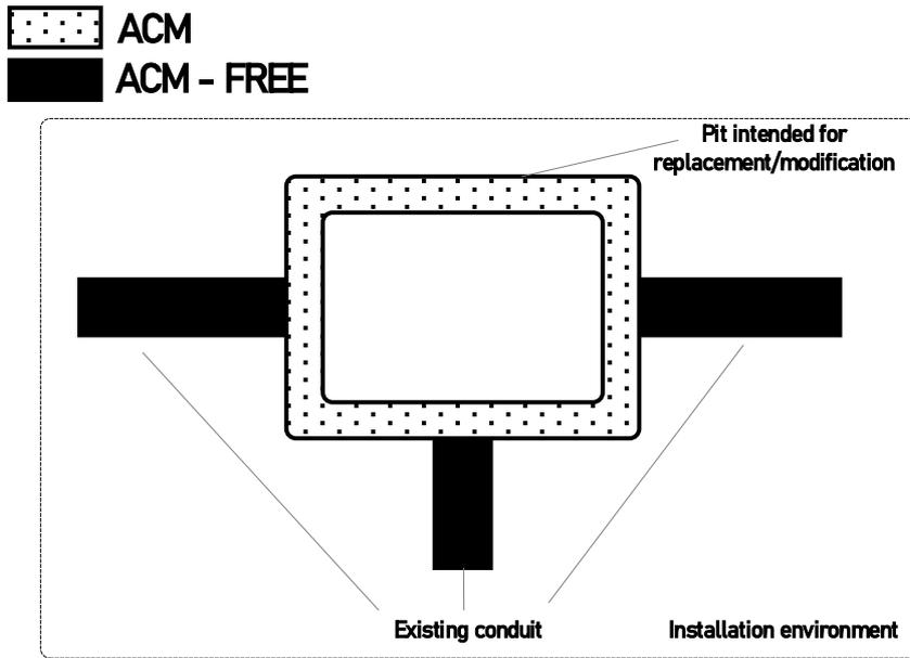
Where the existing pit contains ACM and the linked conduits are ACM-free, the maintenance of the ACM pit shall be handled in accordance with Clause 6.1 and Asbestos management guidelines in MRTS96 *Management and Removal of Asbestos*.
