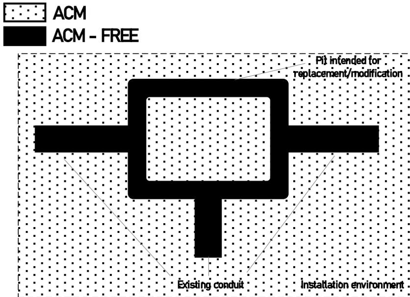
This scenario is mainly about pits and conduits in asbestos contaminated soil but could also include nearby installations suspected to contain asbestos.
