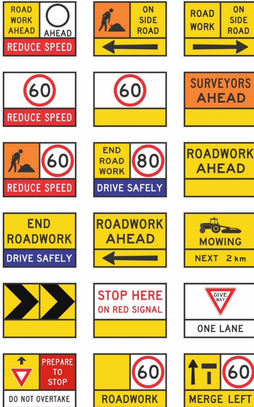
Figure B2 – Additional multi-message sign combination examples with traffic travelling to the right side of the signs
