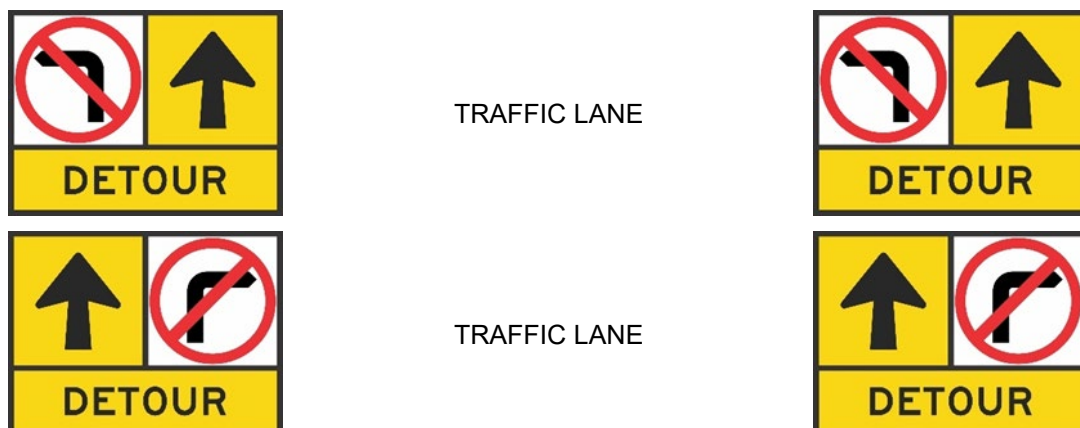
Figure 4.2.2(a) – Example multi-message signs with No Left / No Right Turn prohibition panels
