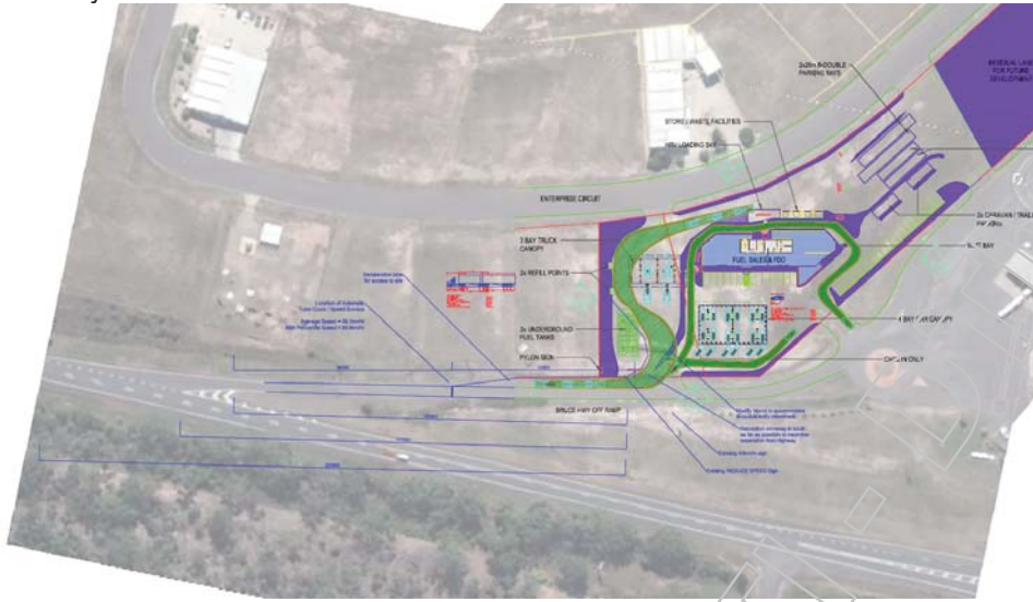
Figure 4 Proposed Auxiliary Left Turn treatment within exit ramp
