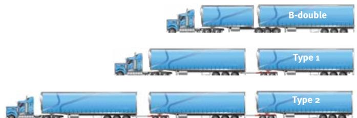
Figure 6: Size difference between B-double, Type 1 and Type 2 road trains
