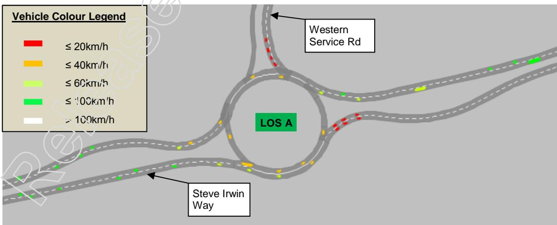
The VISSIM models showed that the proposed configuration at the Pignata Road underpass will operate efficiently in 2031. Typical queuing in both peak periods is shown in Figure 18:
