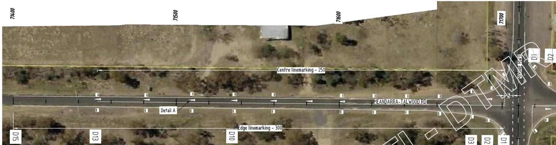
Detail A shall be placed centrally on the lane terminating at the intersection.
