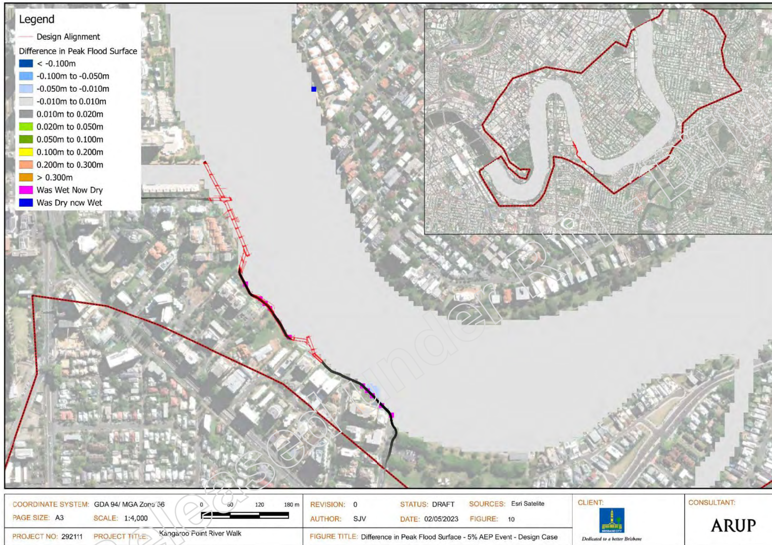
Figure 12: KPRW 5% AEP local peak level afflux
