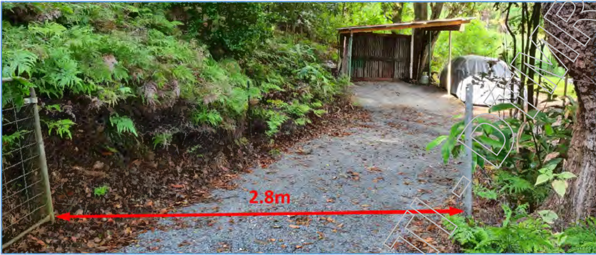
Figure 10: 628 Gate access width.
