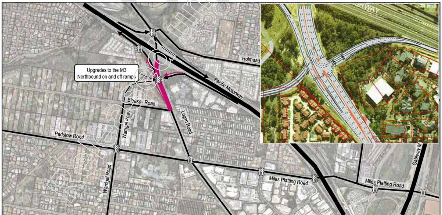
Figure 61 Fat pen sketch of Option 5: Logan Road / Warrigal Road intersection upgrade (2010 BC example)
