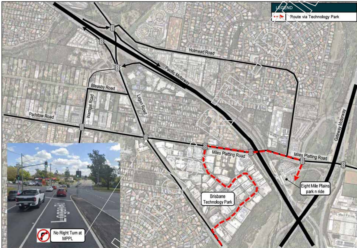
Figure 29 Motorists Travel Through Brisbane Technology Park to Access the Park n Ride
