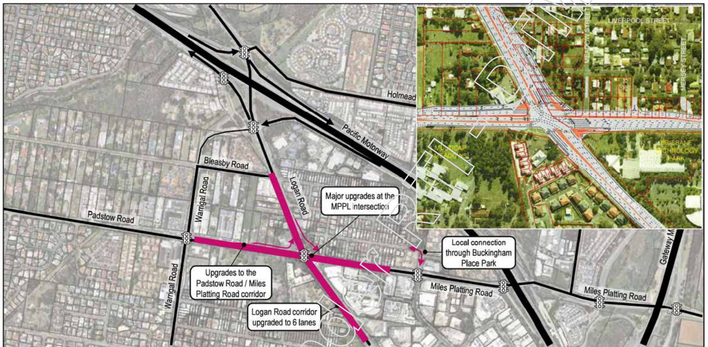
Figure 62 Fat pen sketch of Option 6: MPPL at-grade intersection upgrade (2010 Business Case example)
