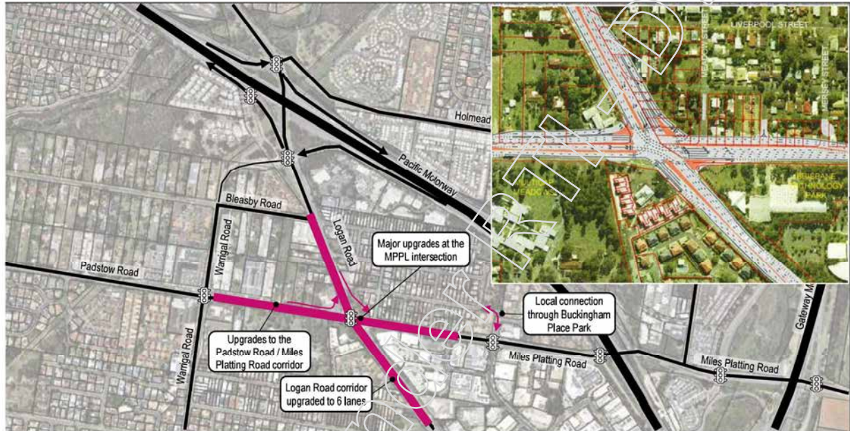
Figure 56 Fat Pen Sketch: MPPL At-Grade Intersection Upgrade (2010 Business Case)
