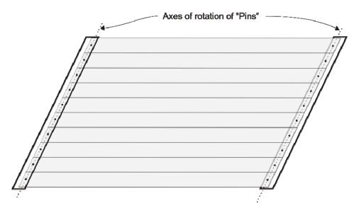
Figure A.15: Orientation of axes of rotation for the "pins" in a skew deck unit bridge
