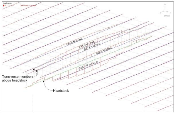
Figure A.3: Axial forces in the headstock and adjacent transverse members
