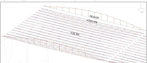
Figure A.13: Typical axial forces in a deck unit span with composite action
