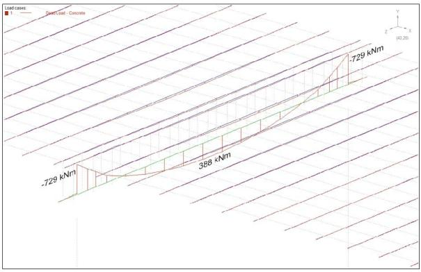
Figure A.6: Bending moments in headstock for corrected model
