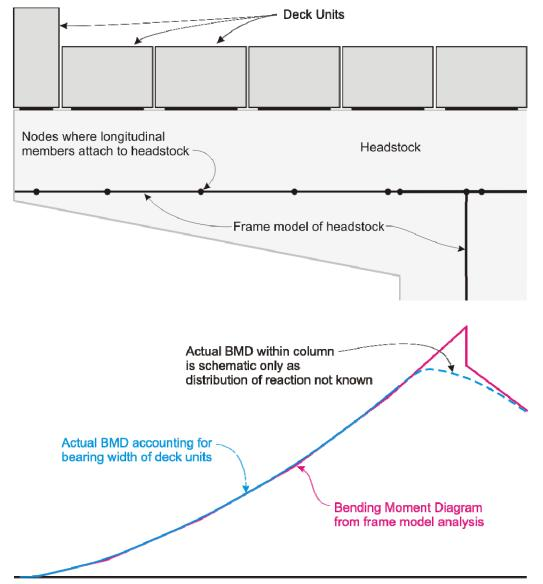
Figure A.17: Bending moment diagrams for the headstock of a deck unit bridge
