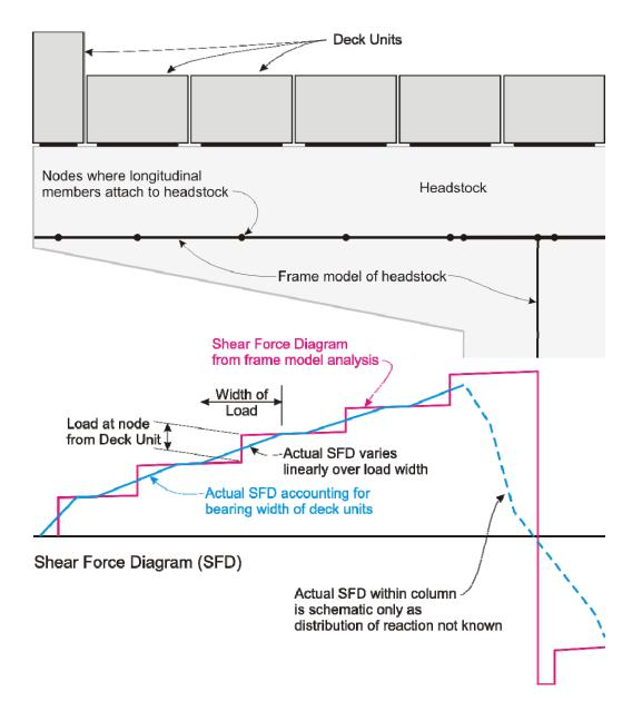
Figure A.16: Shear force diagrams for the headstock of a deck unit bridge
