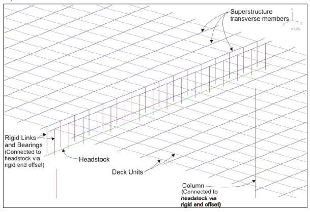
Figure A.1: SpaceGass model at a pier on a deck unit bridge with superstructure vertically separated from the headstock
