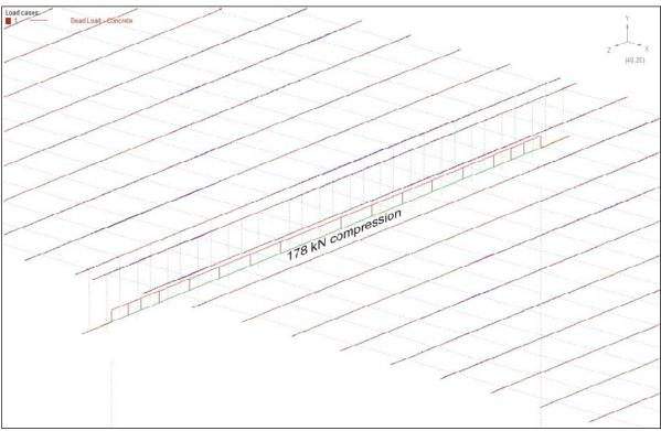
Figure A.7: Axial force in headstock in corrected model
