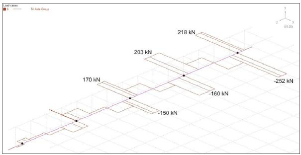
Figure A.9: Horizontal shear in headstock resulting from restrained flexure in deck units
