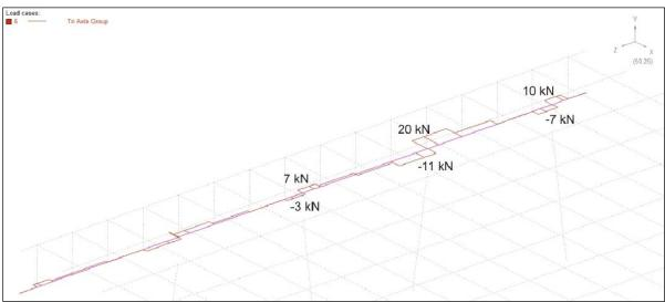
Figure A.11: Horizontal shear in headstock with headstock supported on short piles
