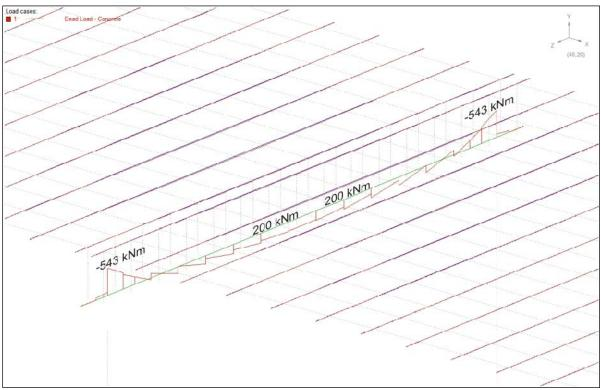
Figure A.5: Bending moments in headstock
