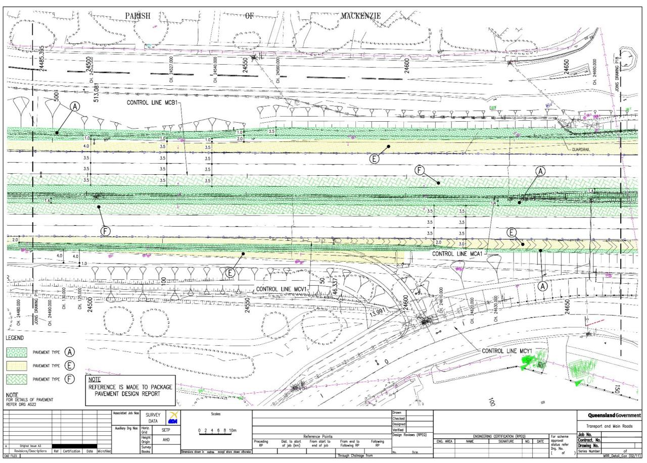
Figure 2.10(d) – Pavement details – generic example 3 – sheet 2 of 2
