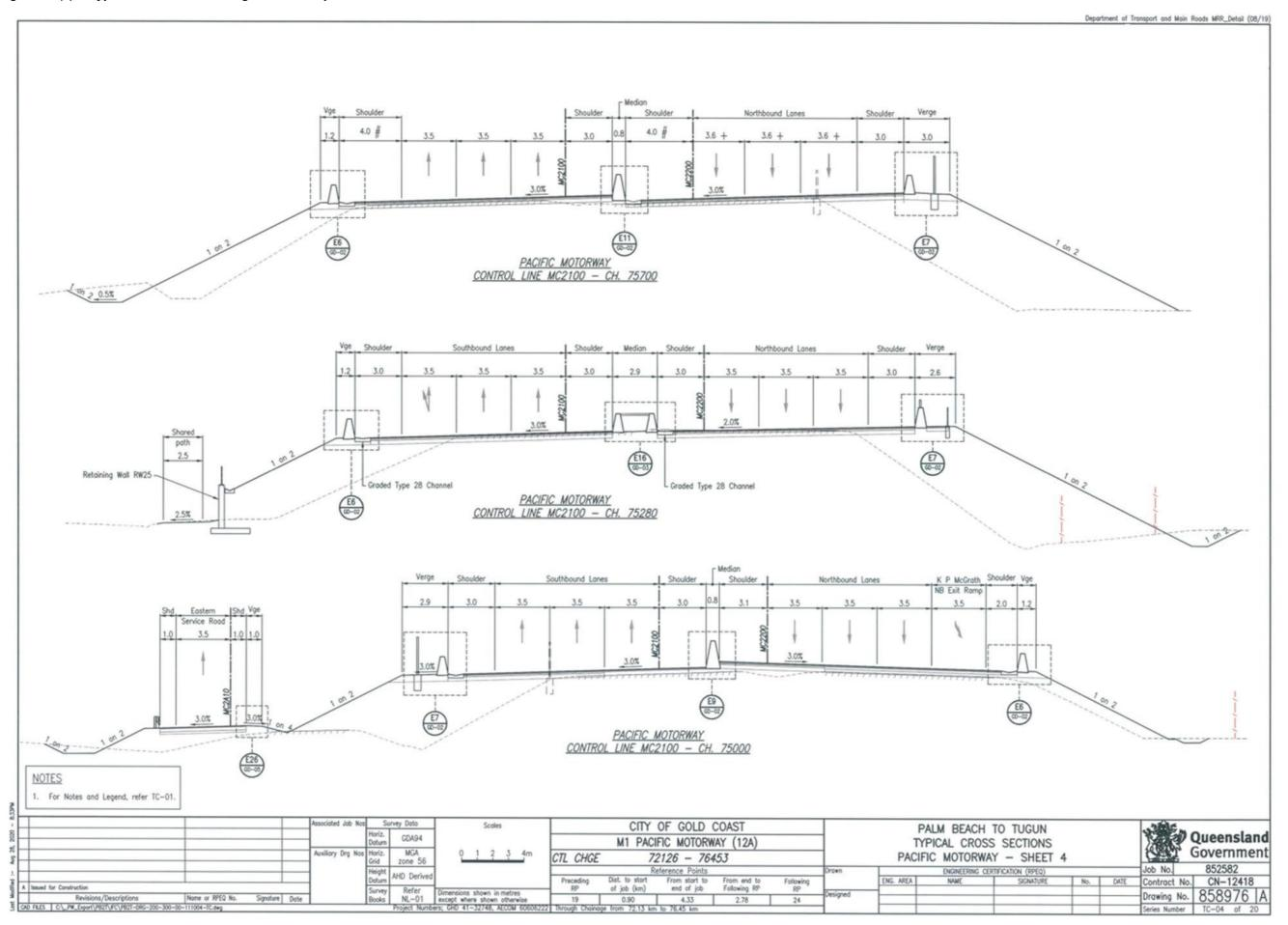
Figure 2.4(b) – Type cross sections – generic example
