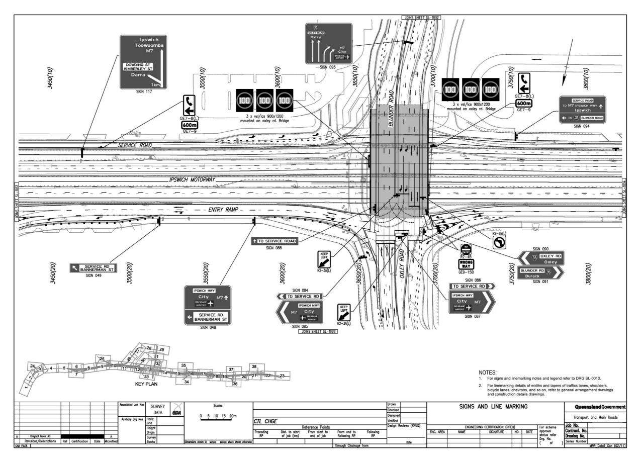
Figure 2.12(h) – Pavement markings and signage – registered example 1
