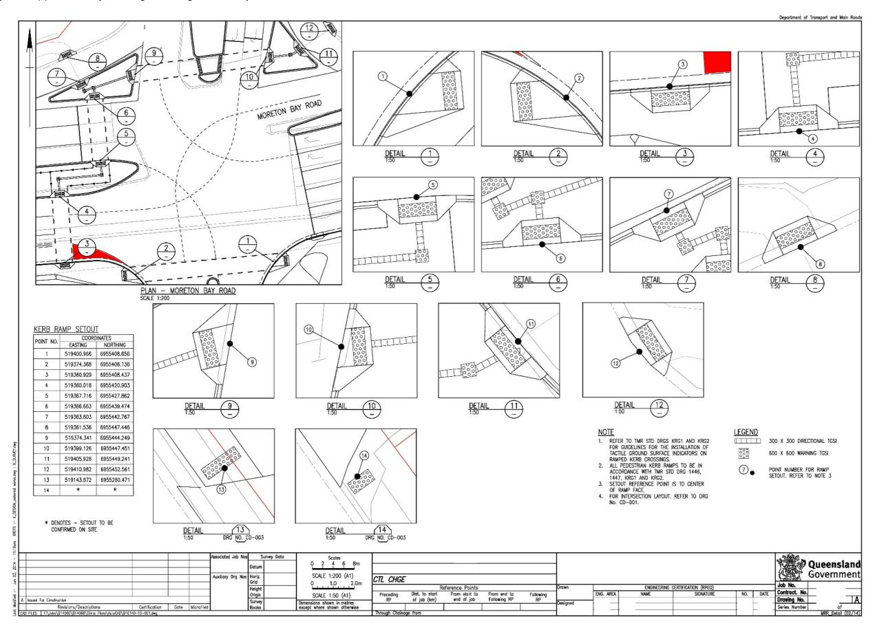
Figure 2.18(d) – Footpath details – generic example
