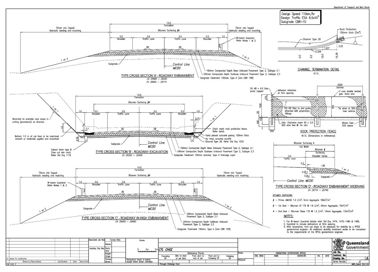
Figure 3.4(e) - Typical cross sections - generic example 1
