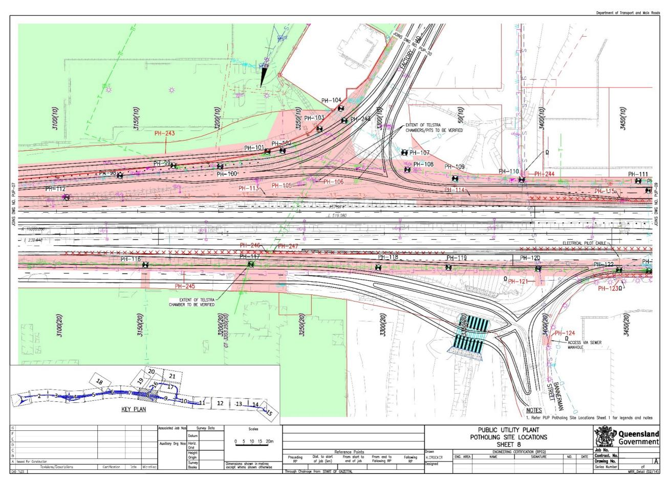
Figure 2.5.2(c) – PUP Potholing and Field Investigation Plans generic example – Sheet 1 of 4
