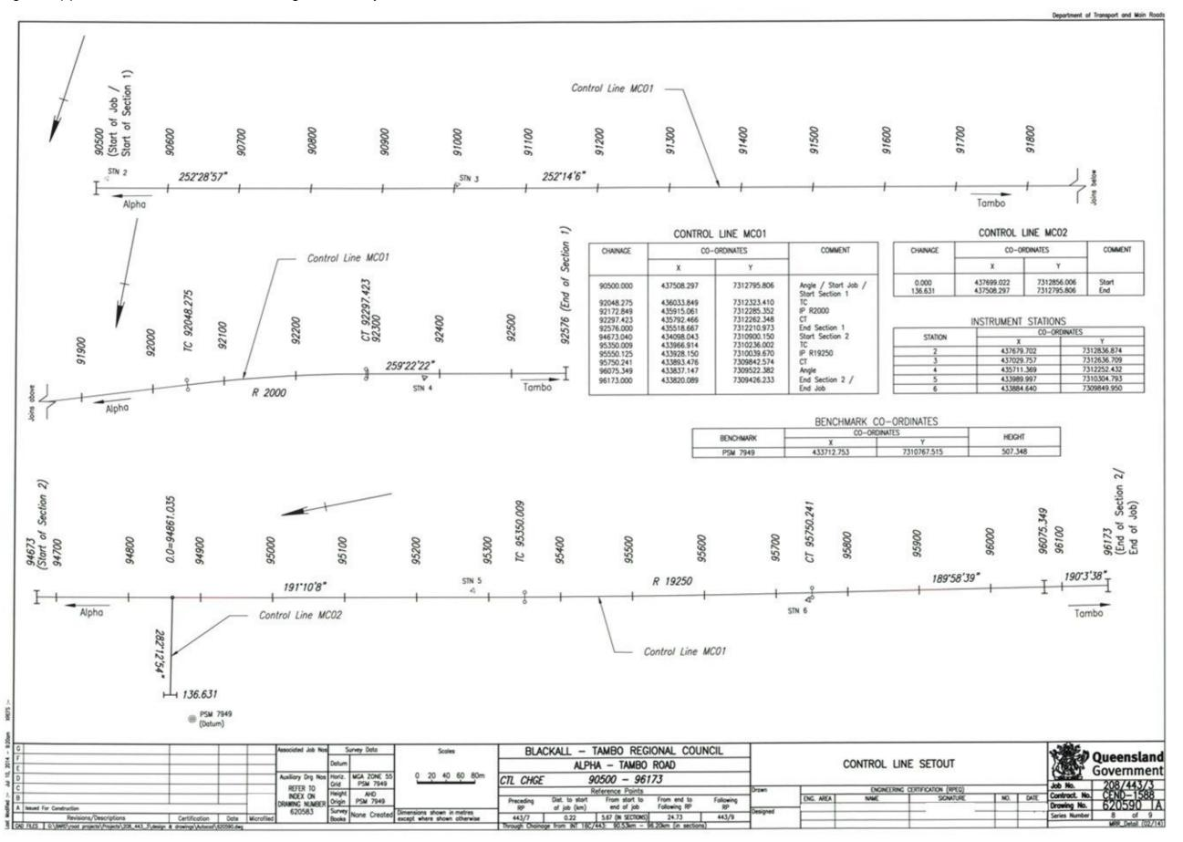
Figure 3.6(e) – Control line set-out and details – registered example 3
