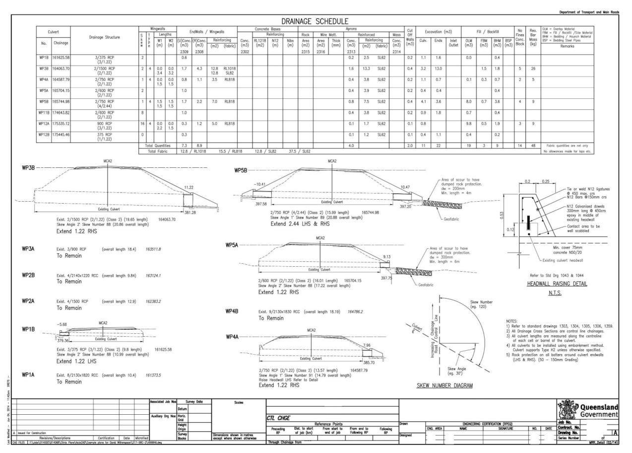
Figure 3.9(d) – Drainage cross sections – registered example 1
