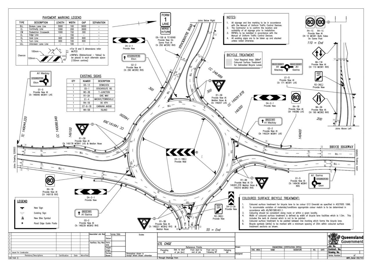
Figure 2.12(b) – Pavement markings and signage – generic example 2
