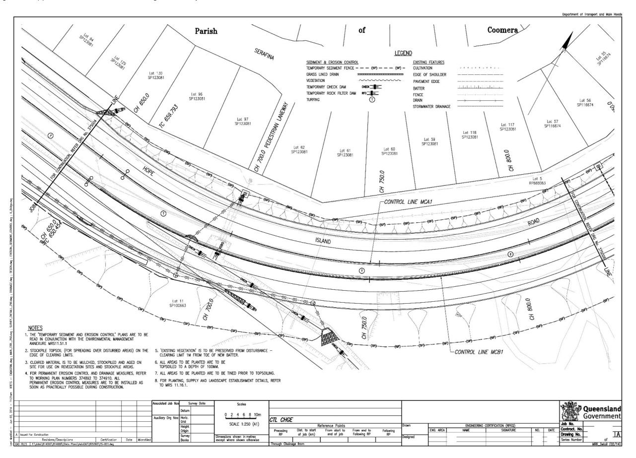
Figure 2.21.2(b) – Erosion and sediment control – generic example 2
