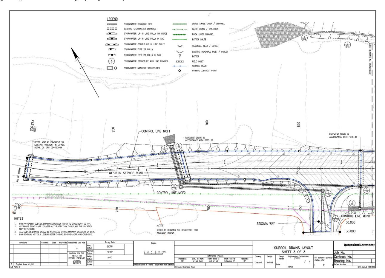
Figure 3.10(g) – Pavement Subsoil Drains Details – generic example
