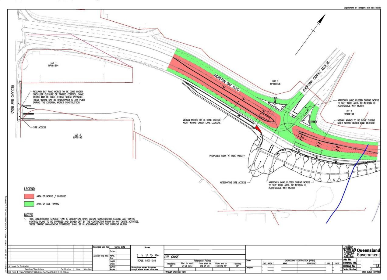
Figure 2.20(c) – Construction staging – generic example 2 – sheet 1 of 2
