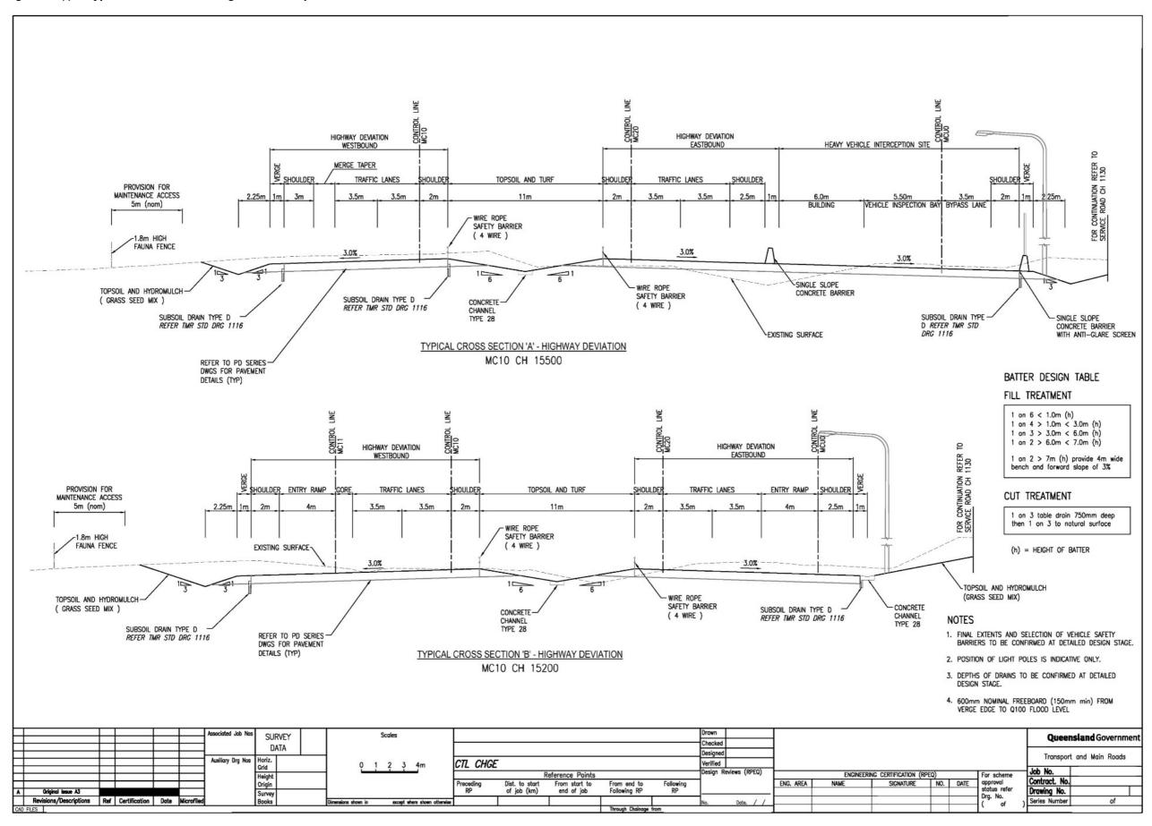
Figure 3.4(g) – Typical cross sections – registered example 1
