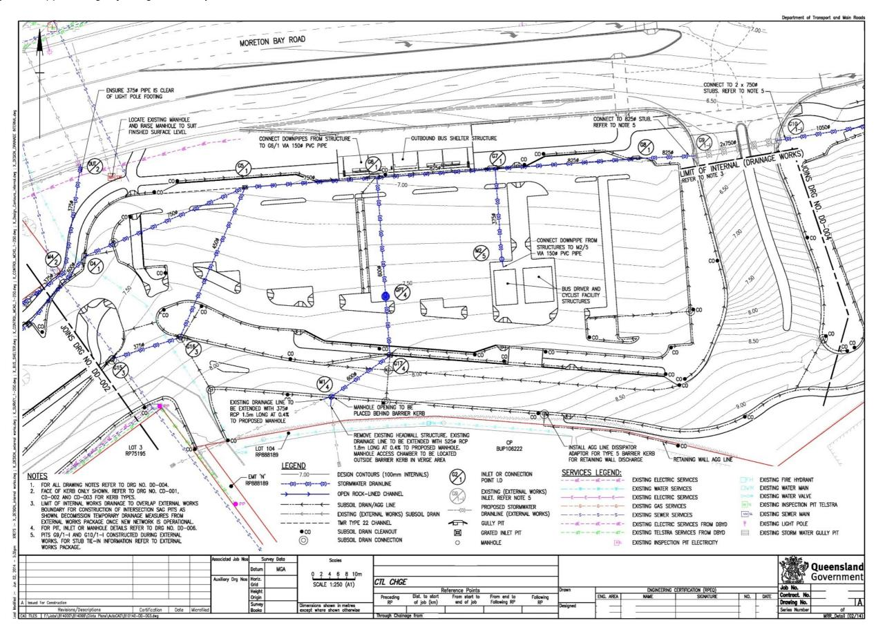
Figure 2.11.1(b) – Drainage layout – generic example 2
