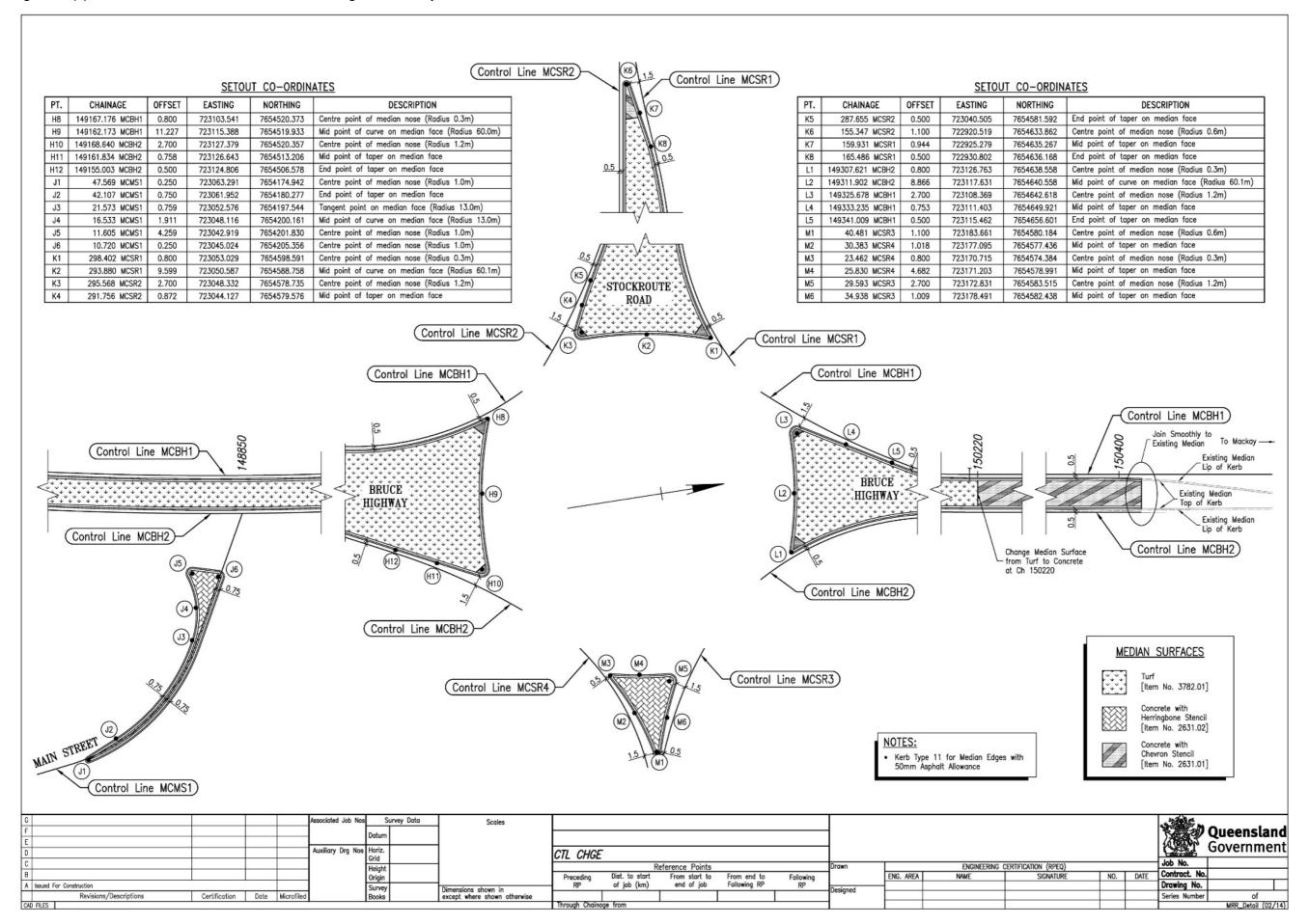
Figure 2.8(c) – Intersection details and set-out tables – generic example 3
