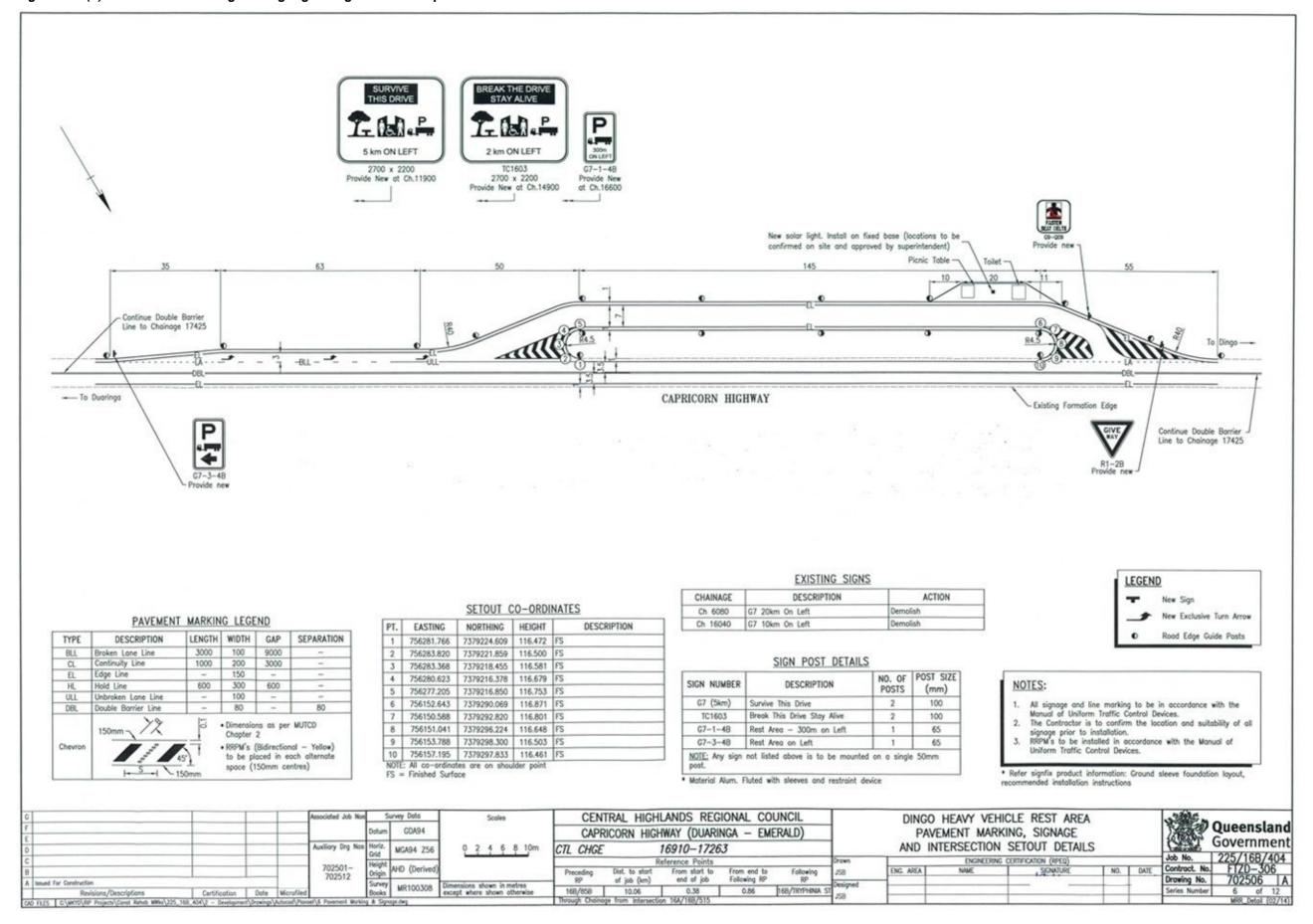
Figure 3.11(e) – Pavement marking and signage – registered example 3
