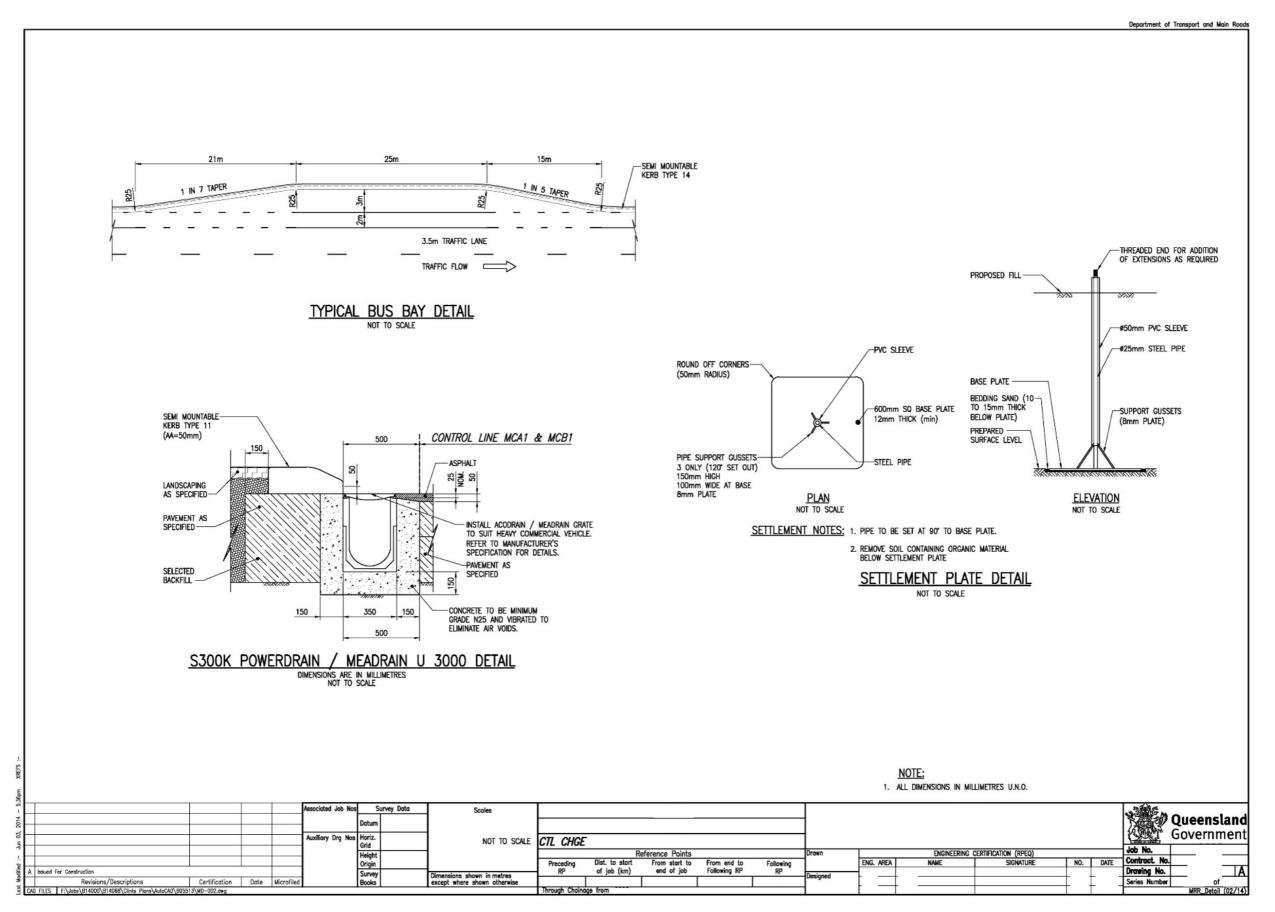
Figure 3.14(d) - Miscellaneous details - generic example 4
