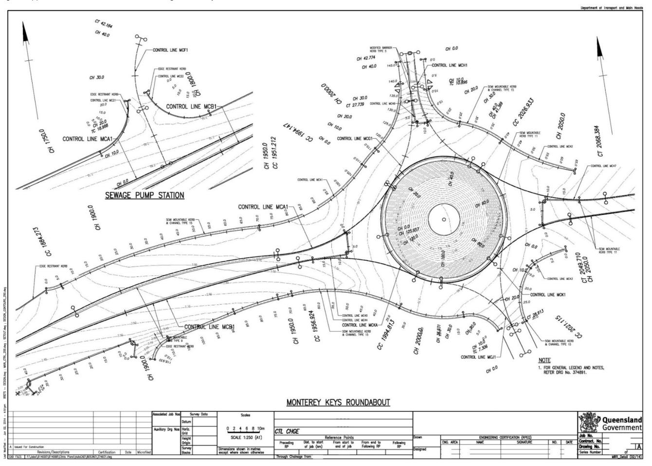
Figure 2.8(d) – Intersection details and set-out tables – generic example 4
