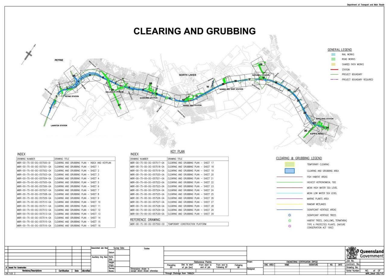
Figure 2.21.1(b) – Clearing and Grubbing – generic example – sheet 2 of 2
