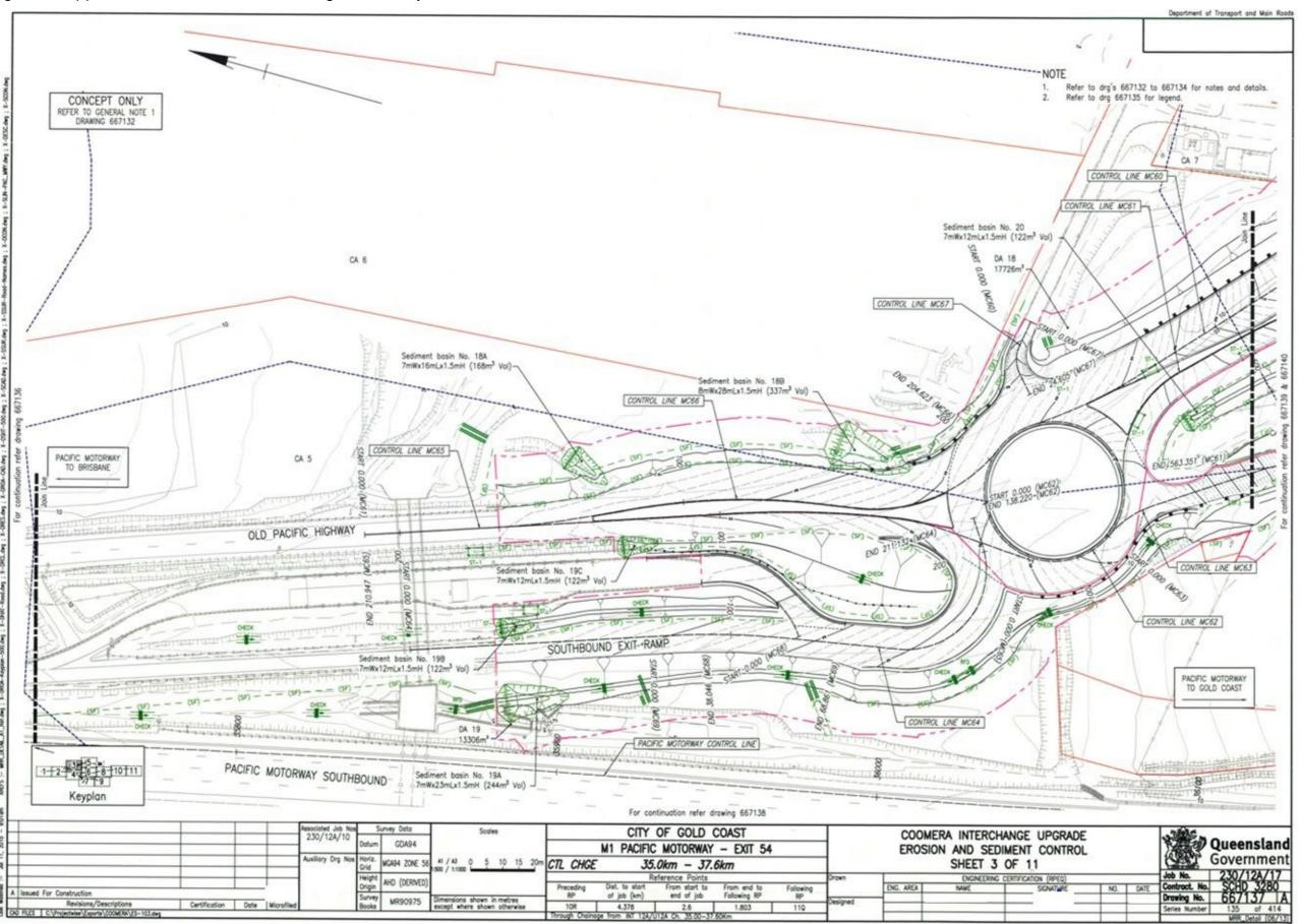
Figure 2.21.2(d) – Erosion and sediment control – registered example 2
