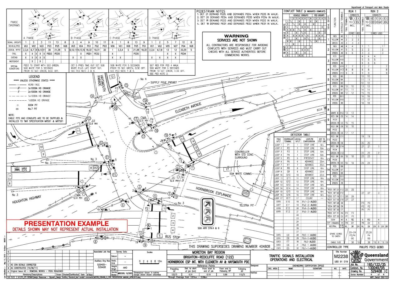
Figure 2.14.4(d) - Traffic Signals - Operations and Electrical - registered example 3
