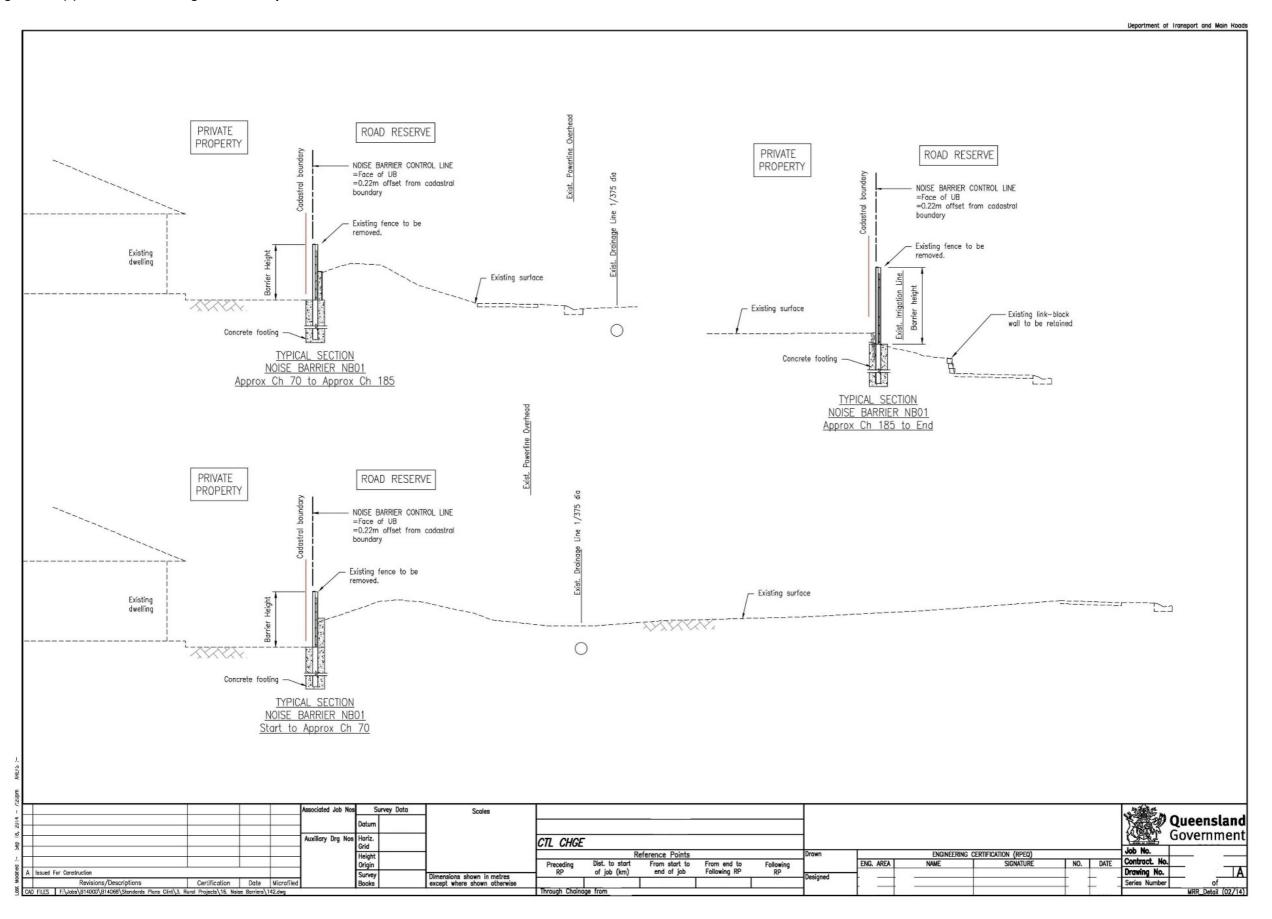
Figure 3.18(d) – Noise barrier – generic example 4
