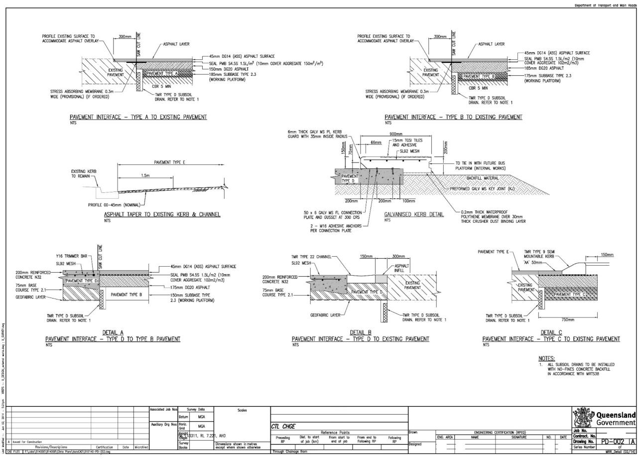
Figure 2.10(c) – Pavement details – generic example 3 – sheet 1 of 2
