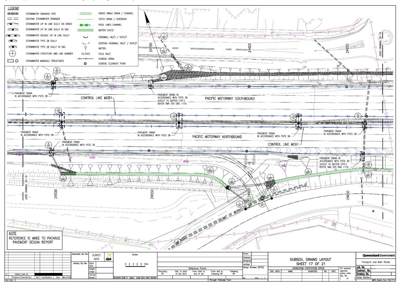
Figure 2.10(f) – Pavement Subsoil Drains Details – generic example
