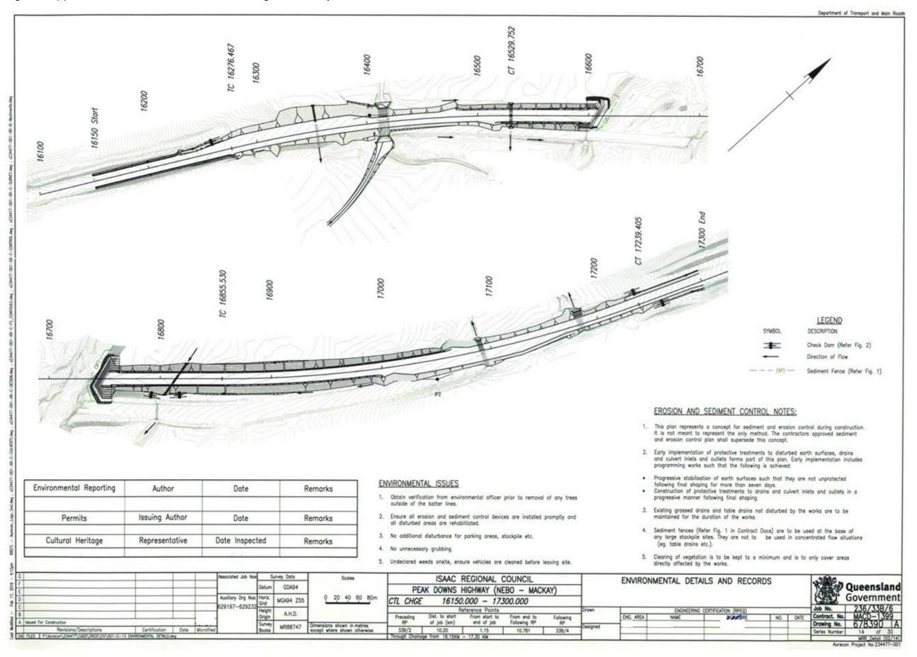
Figure 3.21(d) – Erosion and sediment control details – registered example 3
