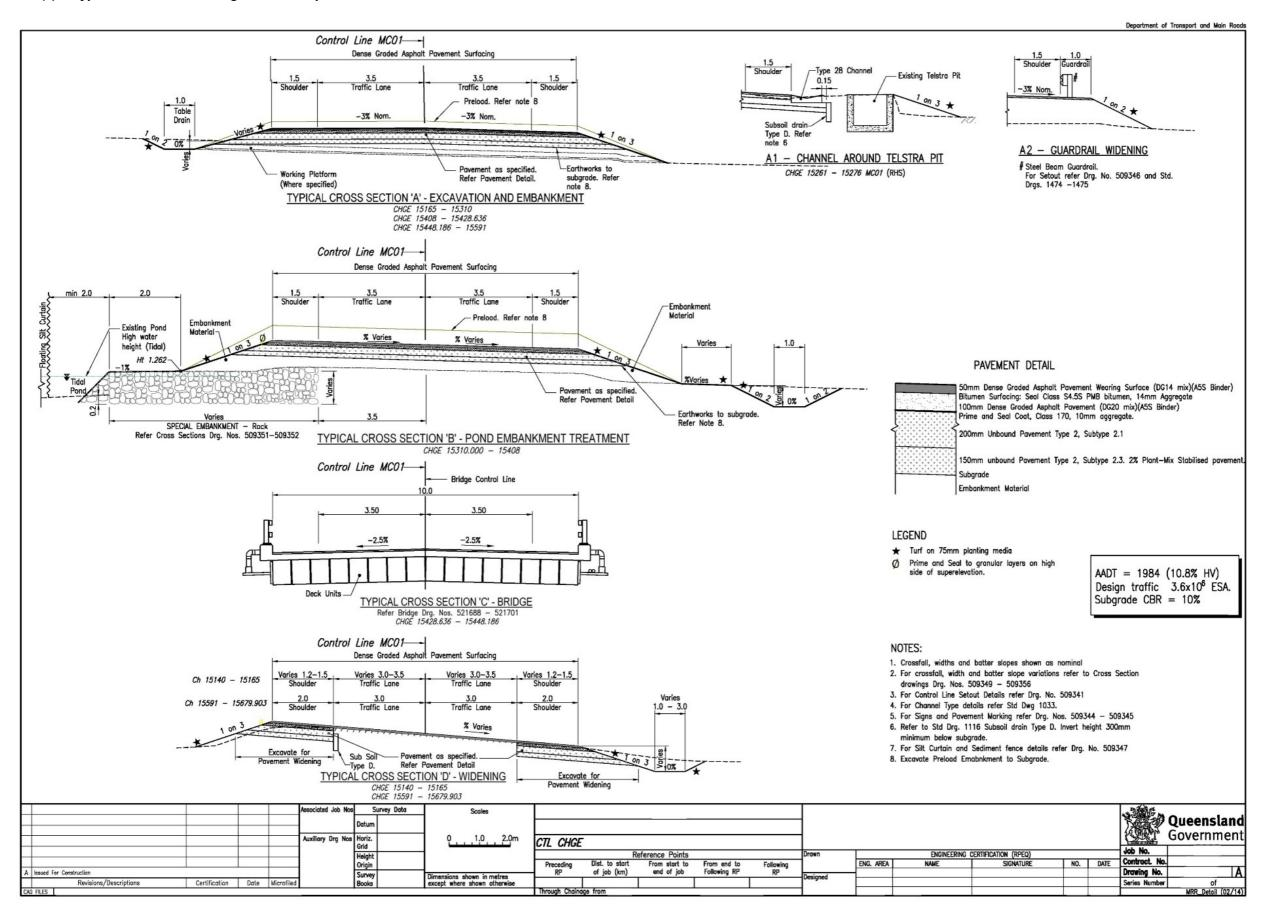
Figure 3.4(f) – Typical cross sections – generic example 2
