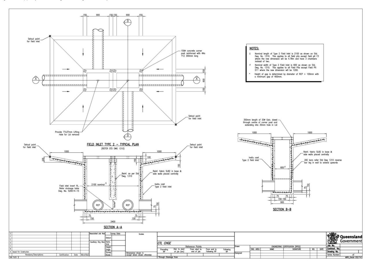
Figure 2.11.4(d) – Specific drainage details – registered example 1
