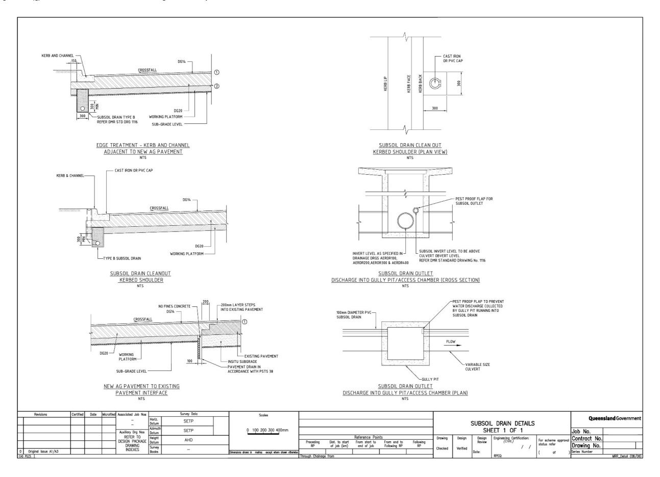
Figure 3.10(h) - Pavement details - registered example 1
