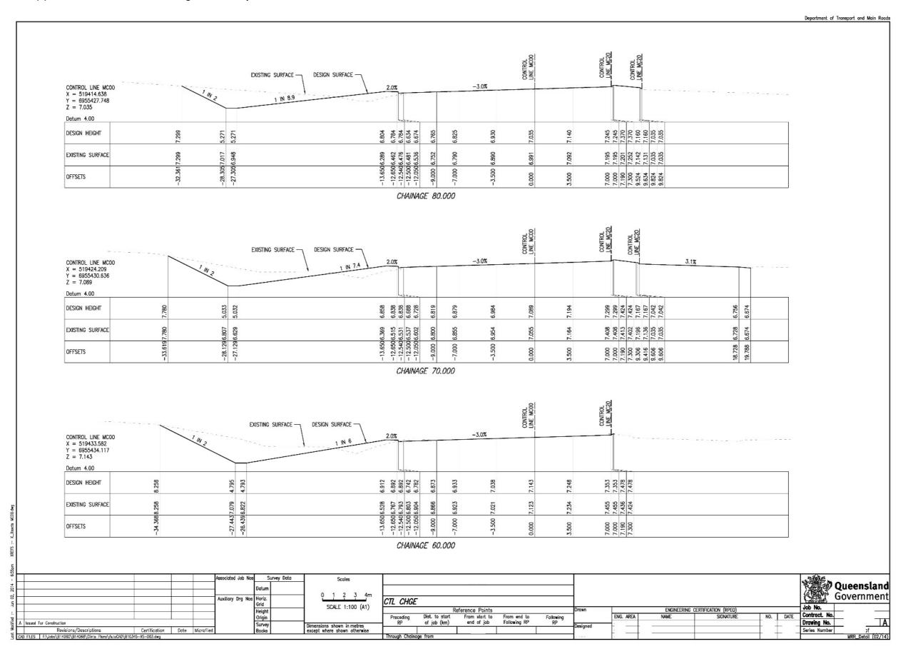
Figure 2.19(c) – Annotated cross sections – generic example 3
