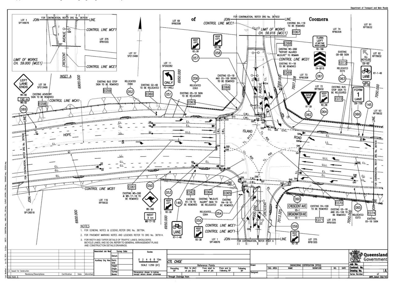
Figure 2.12(d) – Pavement markings and signage – generic example 3 – sheet 2 of 3
