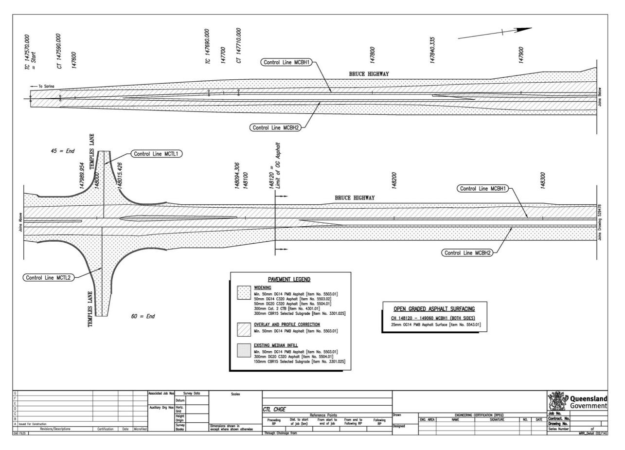
Figure 3.10(b) – Pavement details – generic example 2
