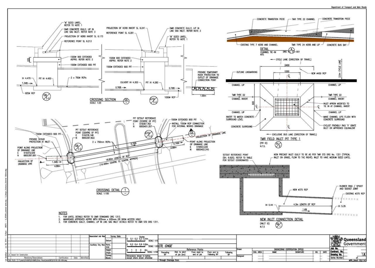
Figure 2.11.4(b) – Specific drainage details – generic example 2
