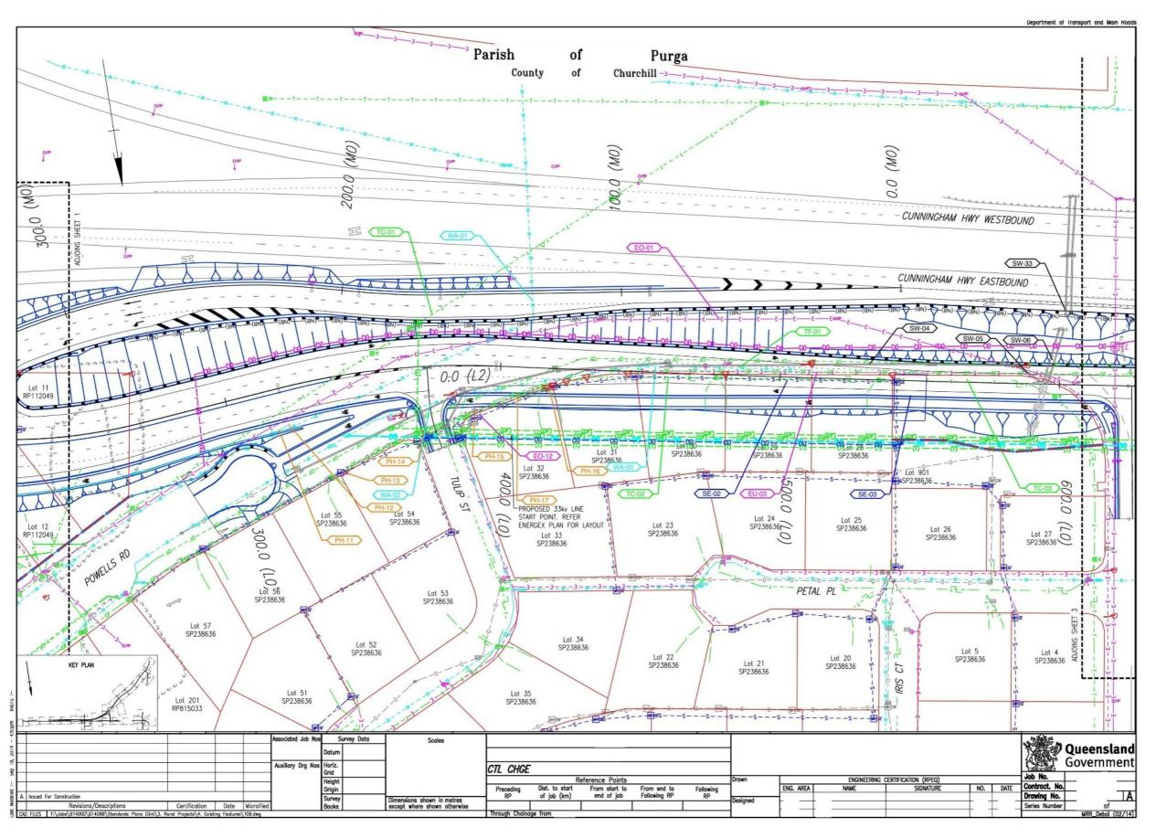
Figure 3.5(c) – Existing features plan with PUP potholing information – generic example sheet 3 of 3
