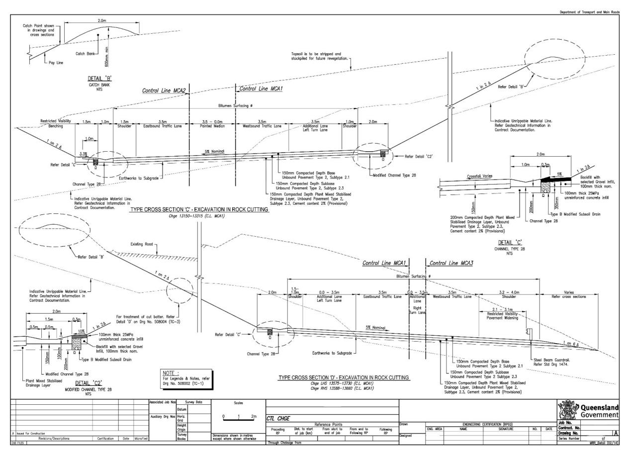
Figure 3.4(c) – Type cross sections – generic example 2
