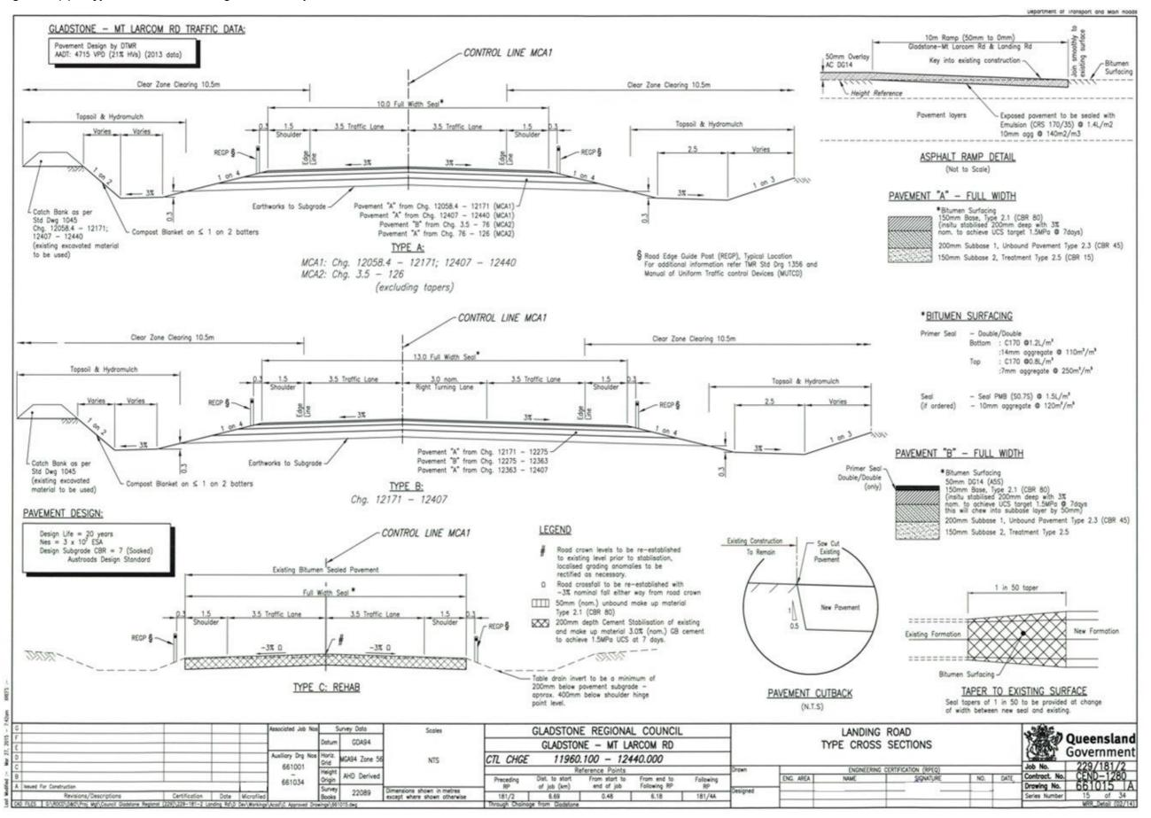
Figure 3.4(i) – Type cross sections – registered example 3
