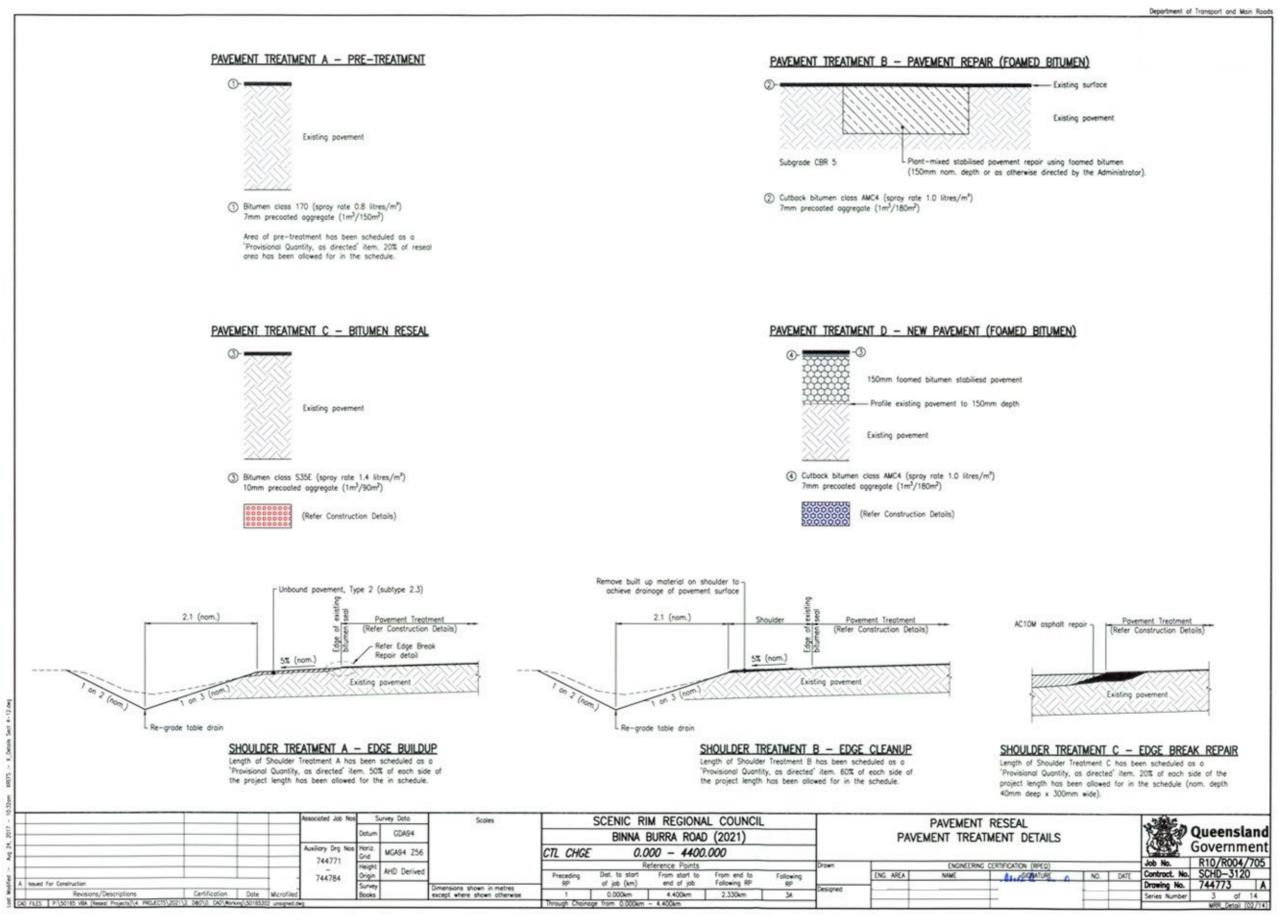
Figure 3.10(j) – Pavement details – registered example 3
