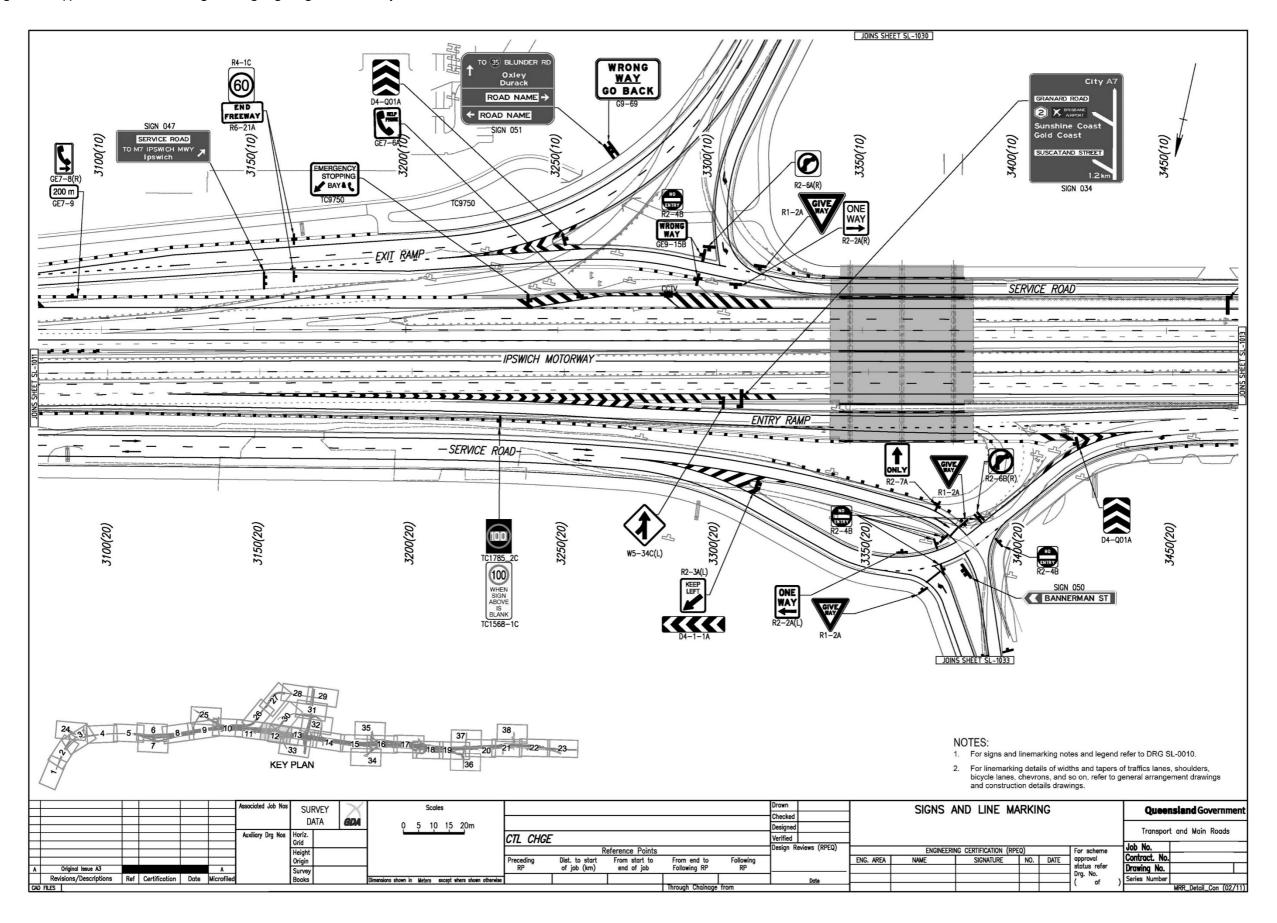
Figure 2.12(g) – Pavement marking and signage – generic example 4 – sheet 2 of 2
