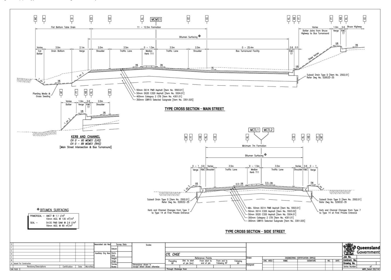
Figure 2.4(c) – Typical cross section details – generic example
