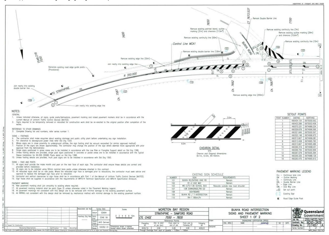
Figure 3.11(f) - Pavement marking and signage - registered example 4
