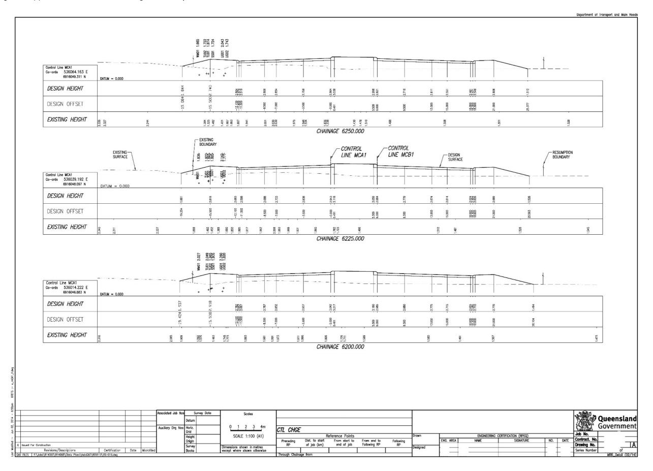
Figure 2.19(b) – Annotated cross sections – generic example 2
