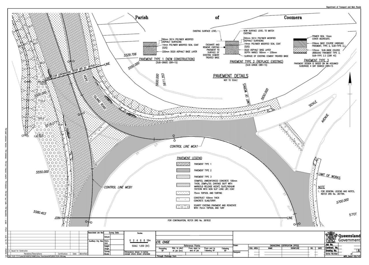
Figure 3.10(c) – Pavement details – generic example 3
