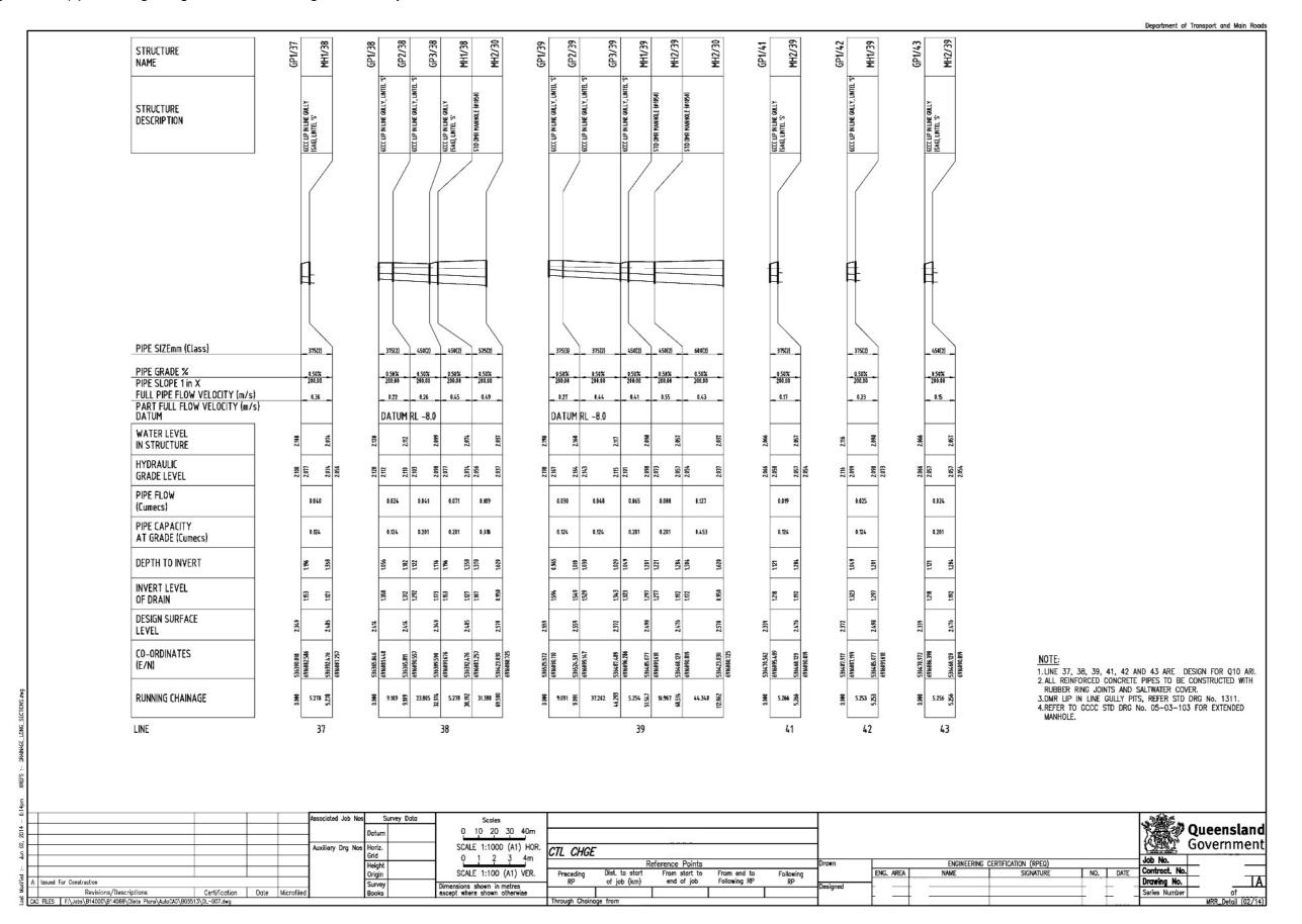
Figure 2.11.3(c) – Drainage longitudinal sections – registered example
