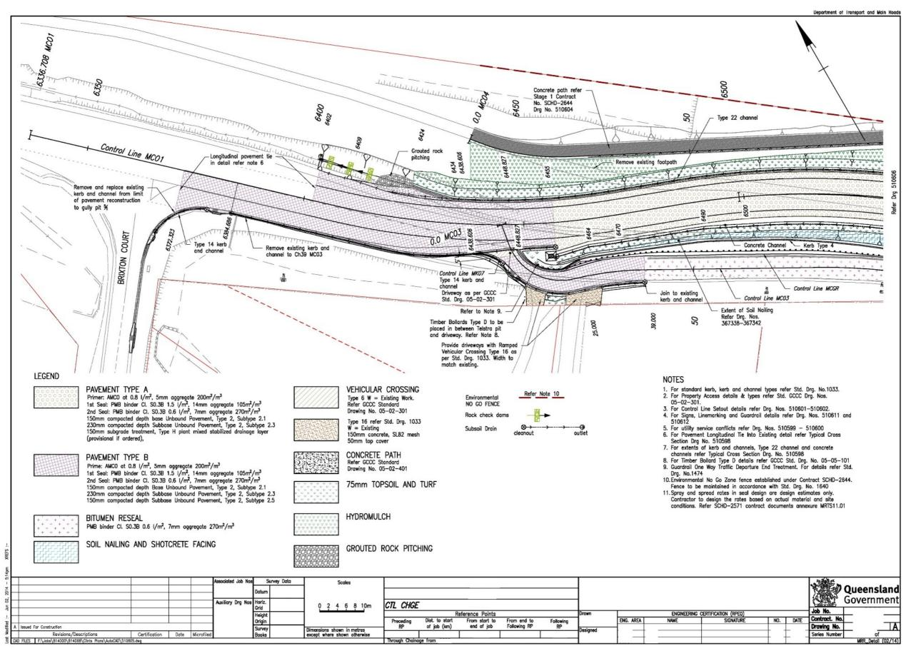
Figure 2.10(b) – Pavement details – generic example 2
