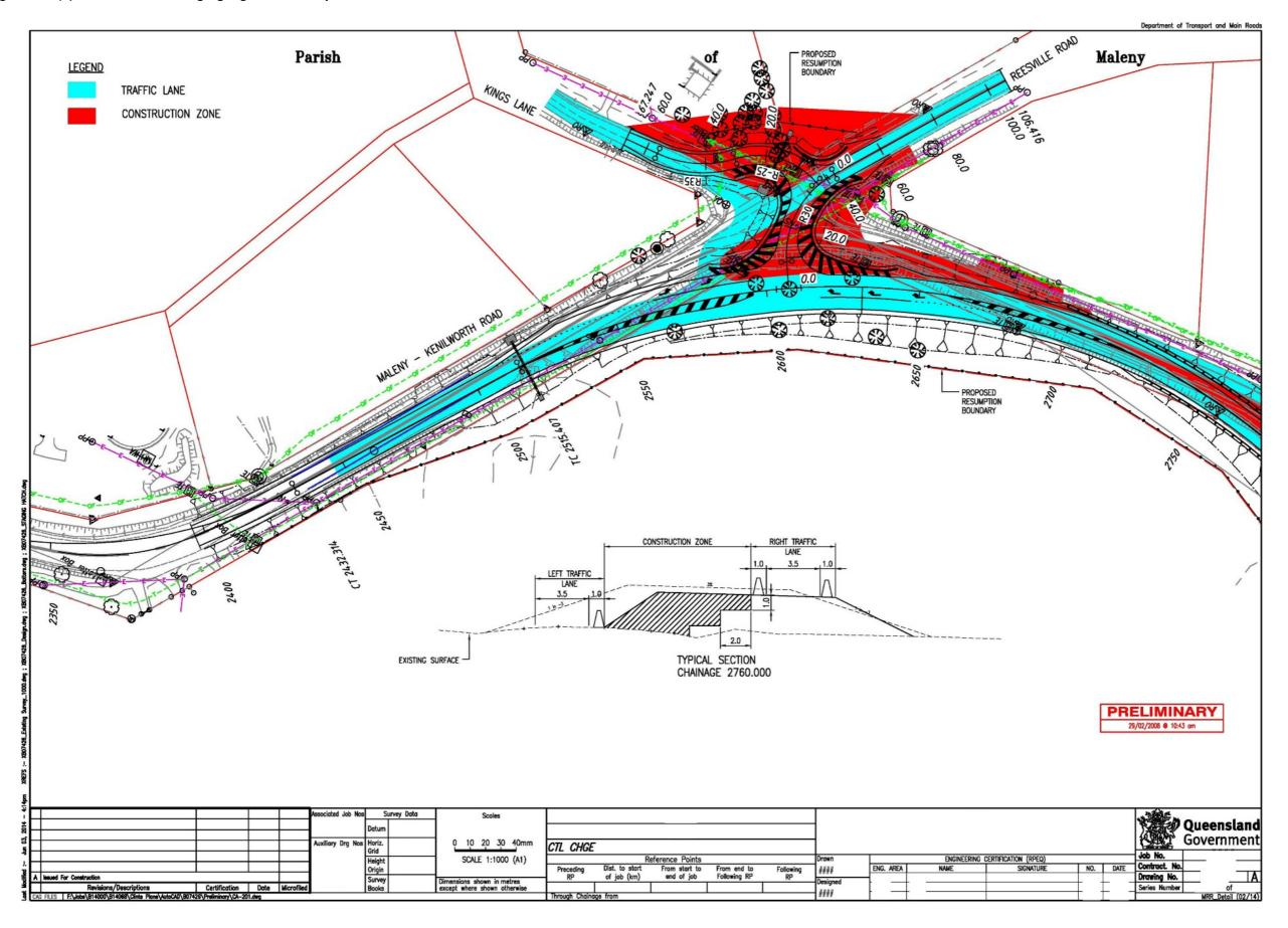
Figure 3.20(c) – Construction staging – generic example 2 – sheet 1 of 2
