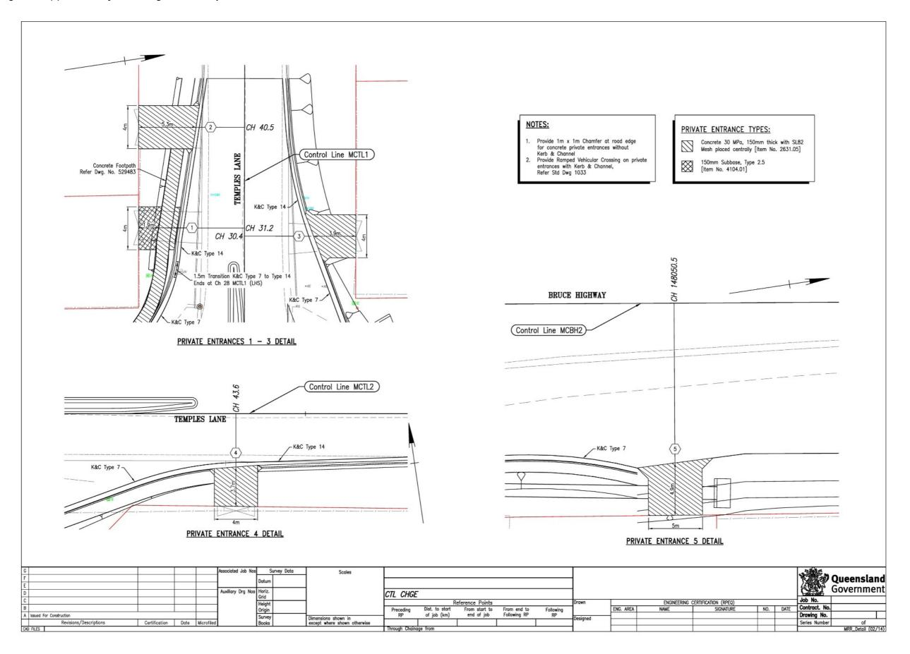
Figure 2.18(b) – Vehicle crossing details – generic example
