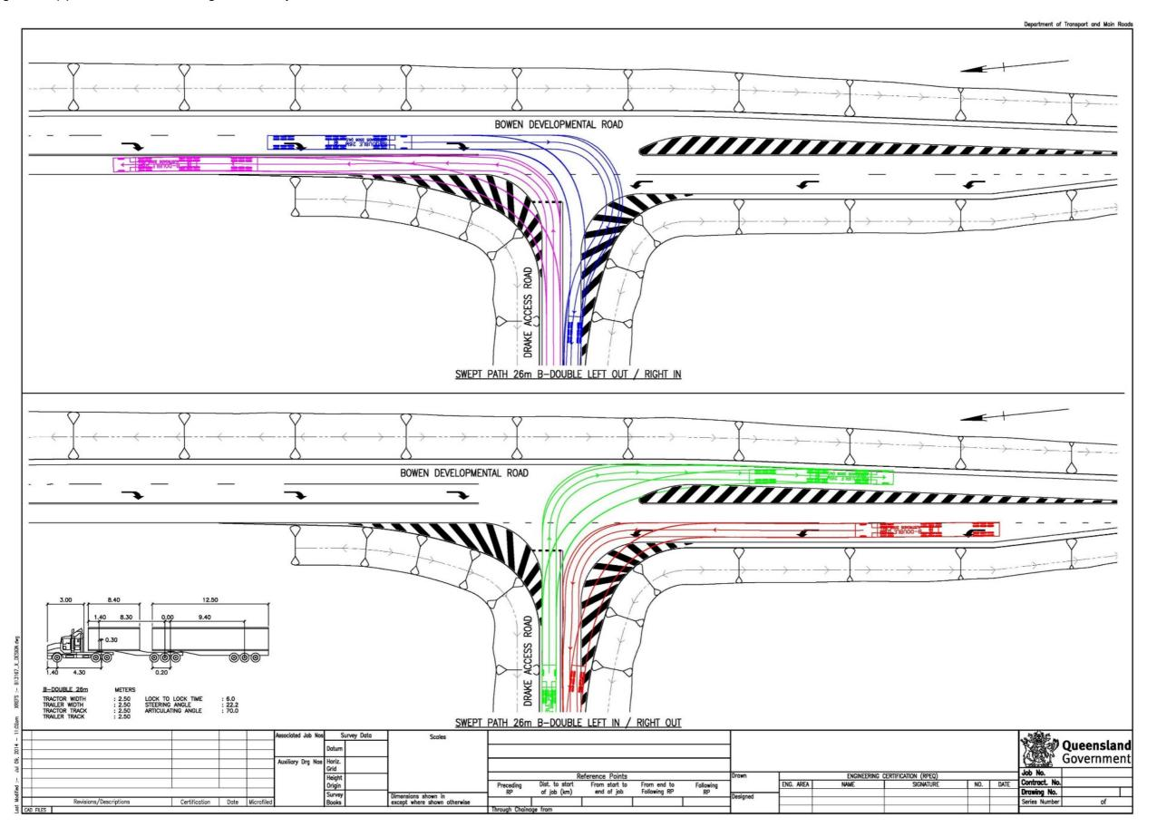
Figure 3.12(e) – Intersection details – registered example
