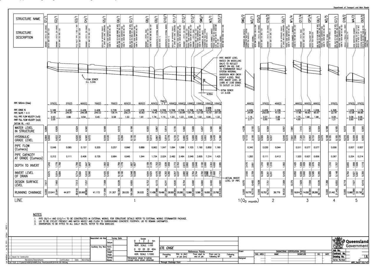
Figure 2.11.3(b) – Drainage longitudinal sections – generic example 2
