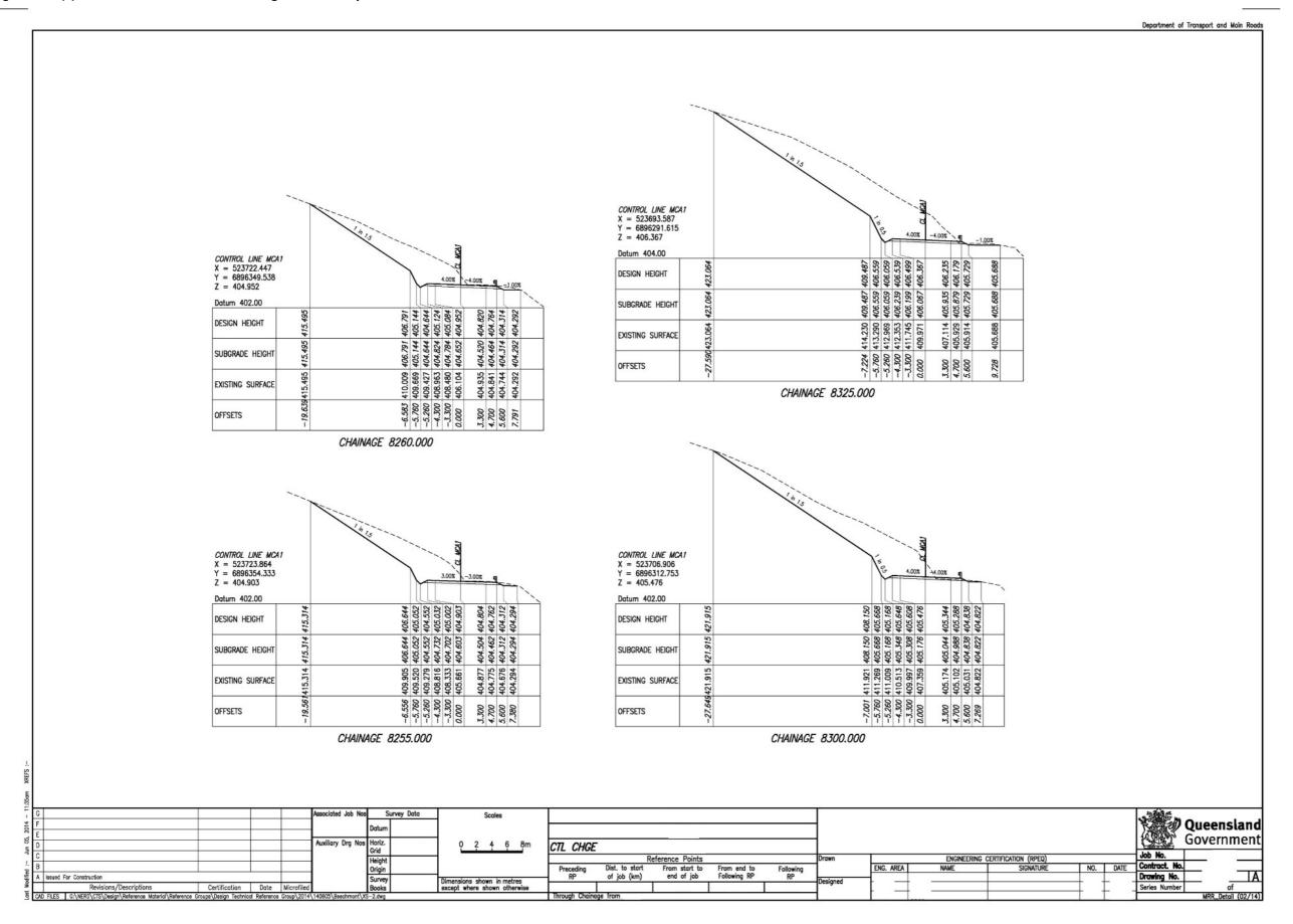
Figure 3.19(b) – Annotated cross sections – generic example 2
