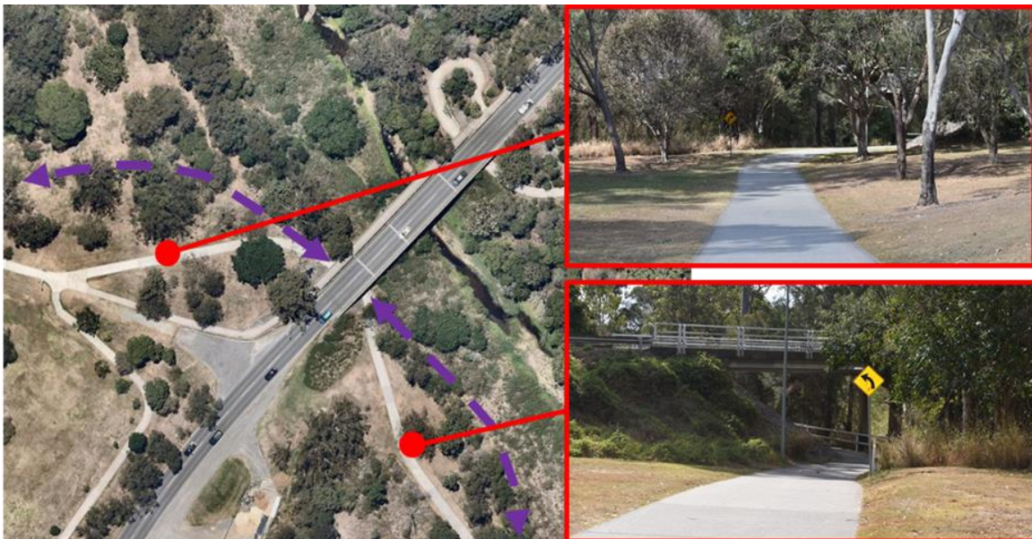
Figure 3.4.2(a) – Curved underpass approach (Kedron Brook Bikeway / Shand Street, Stafford)
