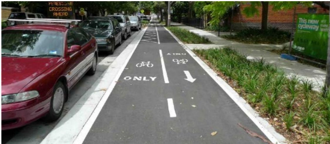
Figure 3.2.6.3(a) – Two-way cycle track, one-step profile – planting separation and pavement contrast, Bourke Street, Sydney
