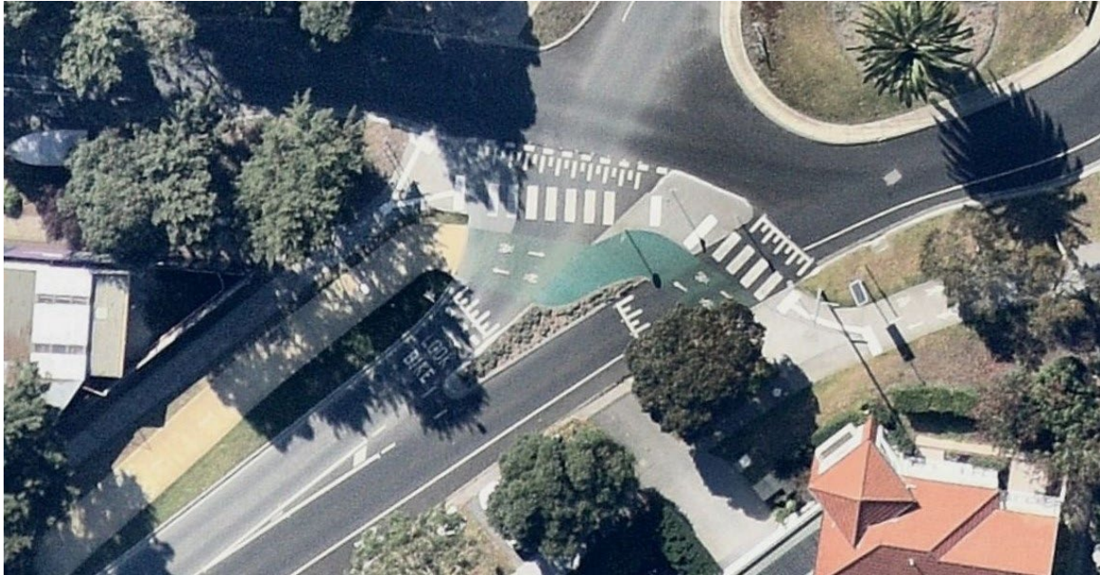
Figure 4.4(a) – Single-lane roundabout, motor vehicle entry and exit ,with two-way cycle track with raised priority crossings and zebra crossings for pedestrian priority, Beach St, Port Melbourne (LTS1)
