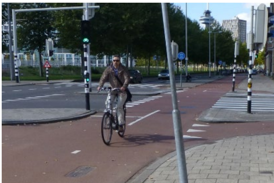
Figure 4.5.2(m) – Dwell-on-green for bicycle traffic at signalised intersection, Rotterdam
