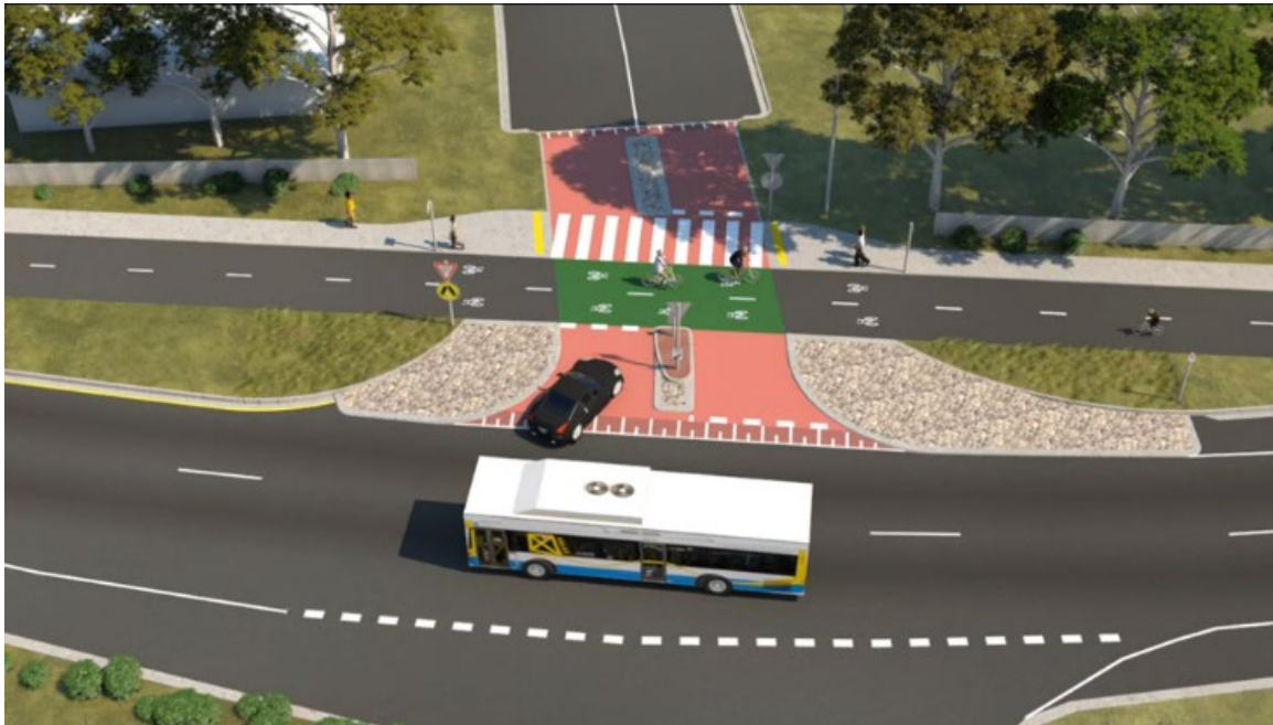
Figure 4.3(c) – Example of two-way cycle track, 5 m buffer from the carriageway at raised priority crossings (different angle)
