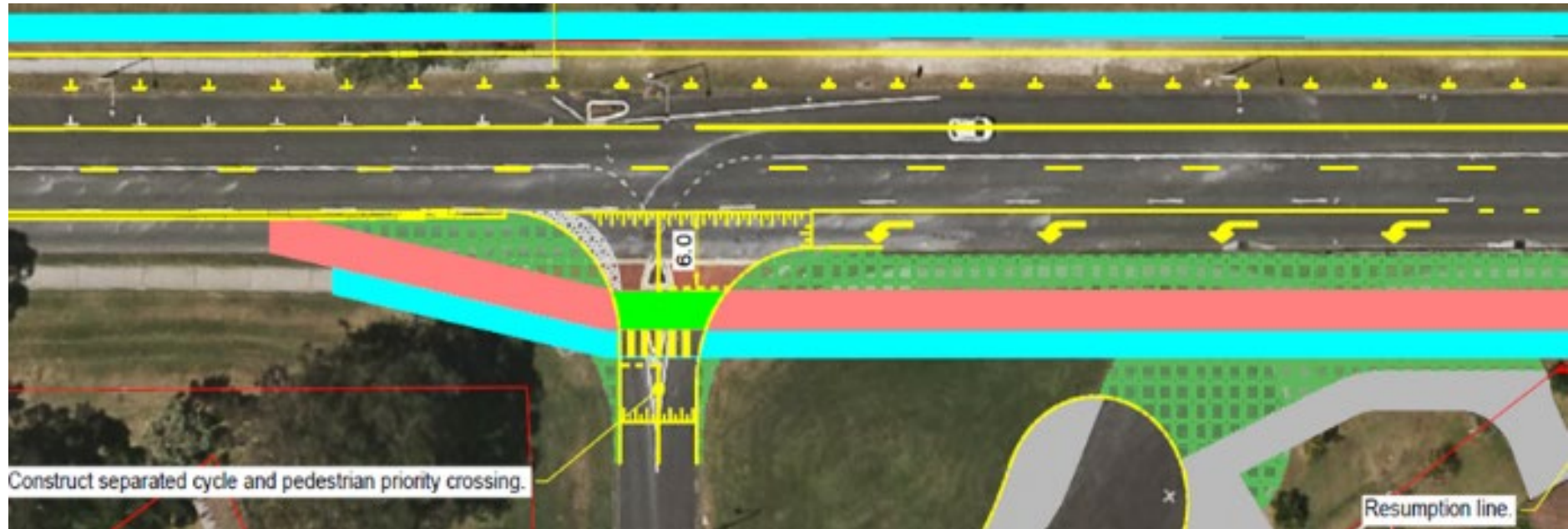
Figure 4.3.1(b) – Concept drawing of two-way cycle track with 6 m storage for exiting vehicles and 3 m buffer for vehicles entering from the added left-turn lane (LTS2)
