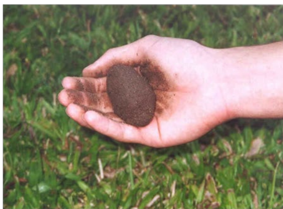
(a) Soil ball almost at sticky point.
