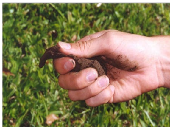
(b) Soil ball being ribboned.
