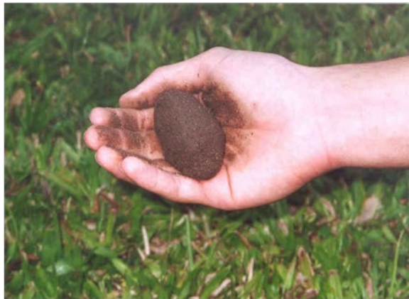
(a) Soil ball almost at sticky point.
