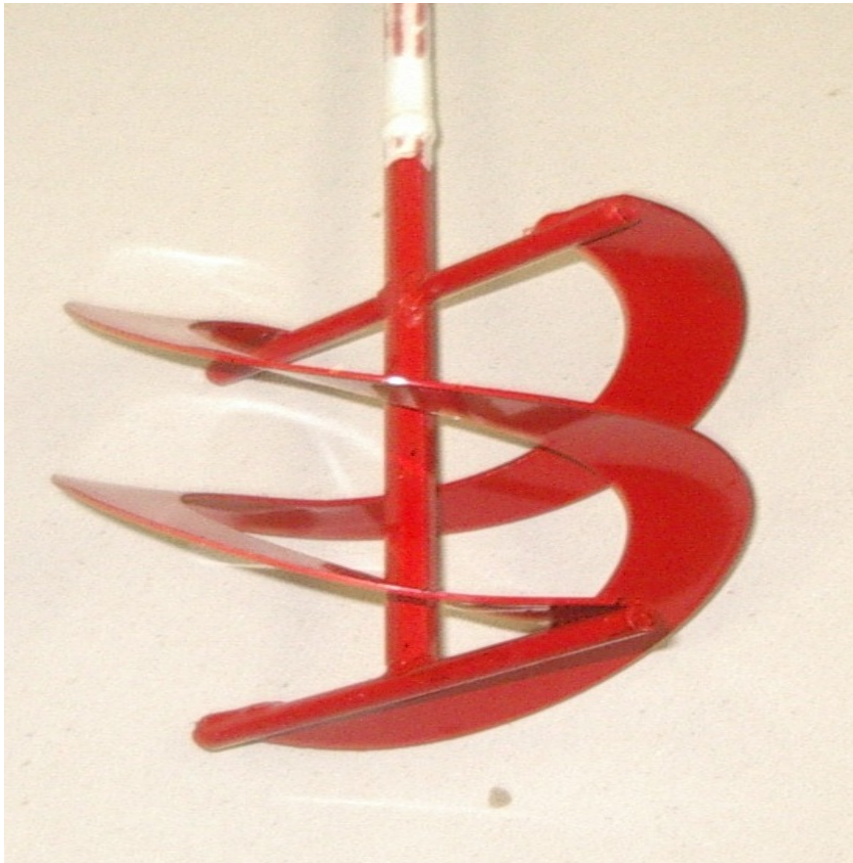
Figure 1 – Mechanical stirrer paddle
