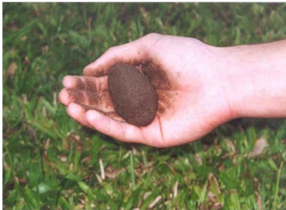
(a) Soil ball almost at sticky point.
