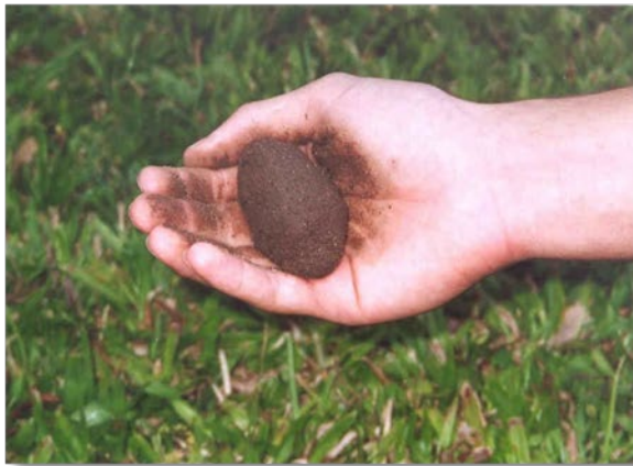
(a) Soil ball almost at sticky point.
