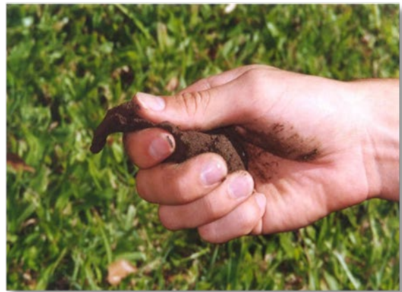
(b) Soil ball being ribboned.
