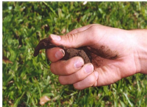
(b) Soil ball being ribboned.
