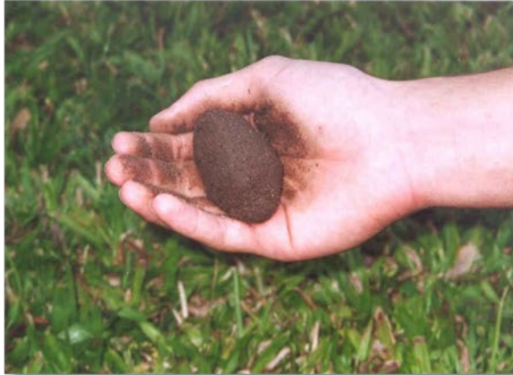
(a) Soil ball almost at sticky point.
