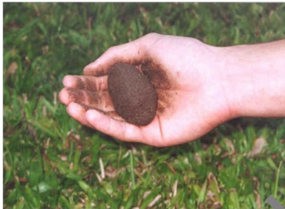
(a) Soil ball almost at sticky point.
