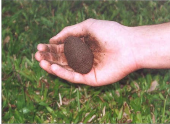
(a) Soil ball almost at sticky point.
