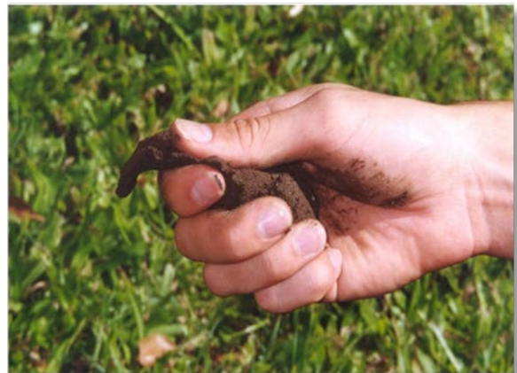
(b) Soil ball being ribboned.
