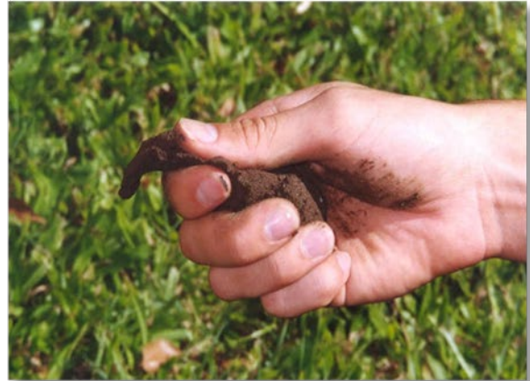
(b) Soil ball being ribboned.
