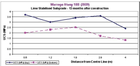
Figure 5.3 – Warrego Highway 18B lime stabilised subgrade – 13 months after construction
