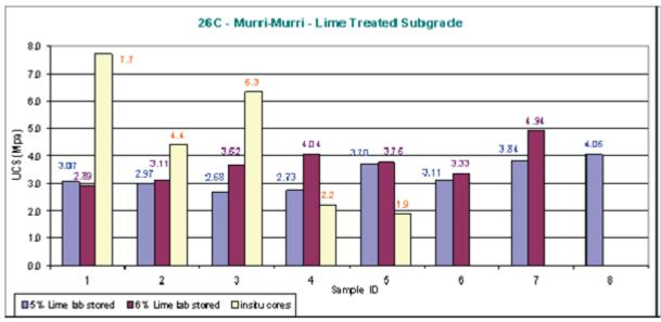
For the 20 cores tested, all results were above 2.0 MPa except for one. It was noted that the exception had the largest length to diameter ratio of all cores.
