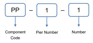
Figure 5.1.3(d) – Short BIM object code example for a precast pile at an abutment
