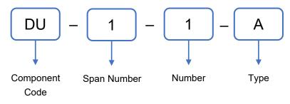
Figure 5.1.3(c) – Short BIM object code example for a precast pile at a pier
