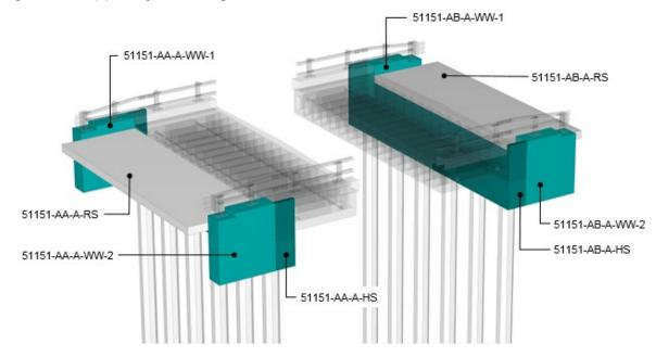
Figure 5.2.2.2(a) – Object naming convention for abutments
