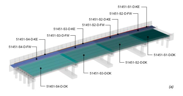
Figure 5.2.3.2(b) – Naming convention for bridge deck objects
