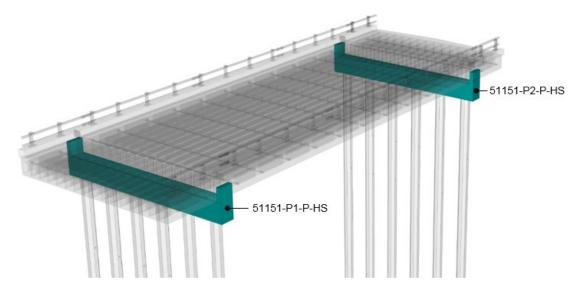
Figure 5.2.2.3(b) – Object naming convention for piers with columns
