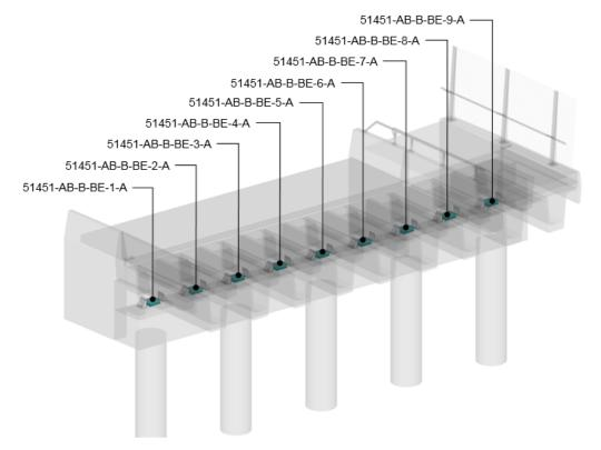
Figure 5.2.2.4(b) – Object naming convention for bearings on abutments
