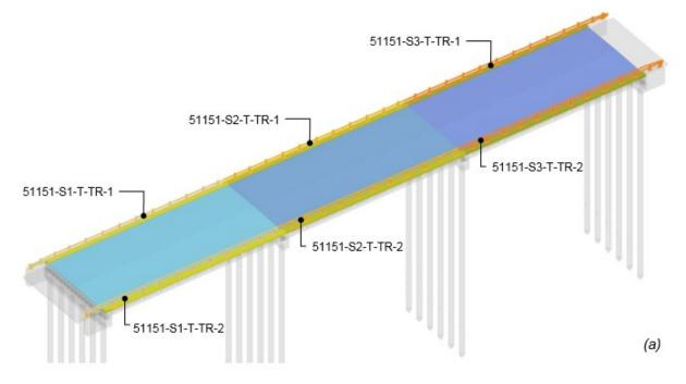
Figure 5.2.3.3 – Naming convention for bridge barrier objects
