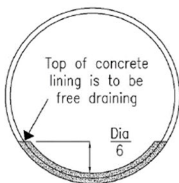
Figure 3.6.10(b) – Culvert lining details
