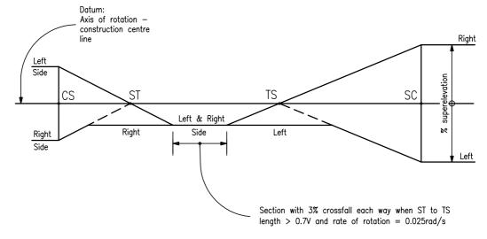
Case 2: <u>REVERSE TRANSITIONED CURVES WITH LENGTH OF INTERVENING TANGENT > 0.7V</u> (Corresponds to the standard case in Figure 11.1)
