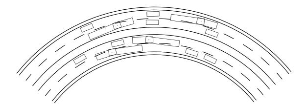
Figure 11.4 Examples of Heavy Vehicle Operation on Multi-lane Roads with Insufficient Curve Widening
