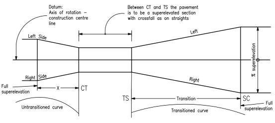
General treatment of similar curves when distance between tangent points < 3V metres (V in km/h)
