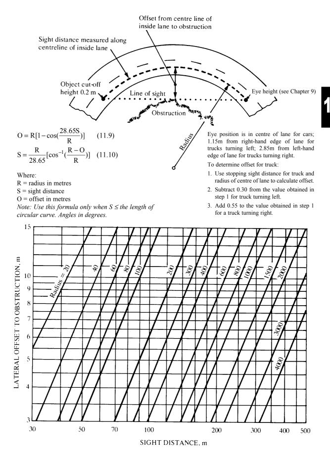
Figure 11.6 Horizontal Stopping Sight Distance for Type F Restriction to Visibility (Reaction Time = 2.5 seconds)
