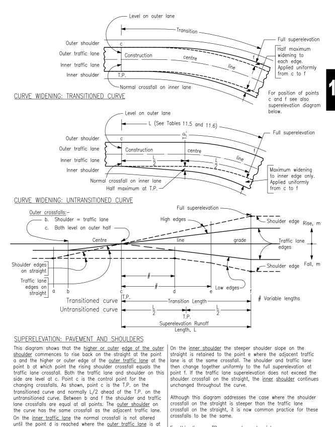
For this diagram TP = curve tangent point TP = the TS and ST points on a transitioned curve = the TC and CT points on an untransitioned curve.
