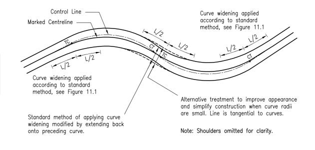
Figure 11.5 Application of Curve Widening on Closely Spaced Reverse Untransitioned Curves
