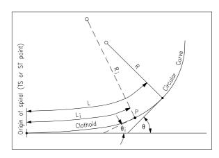
Figure 11A.1 Clothoid Spiral Transition Curve
