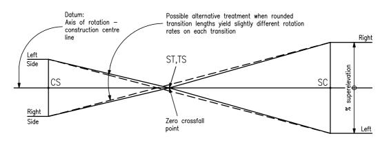
Case 1: REVERSE TRANSITIONED CURVES WITH COMMON POINT OF TANGENCY
