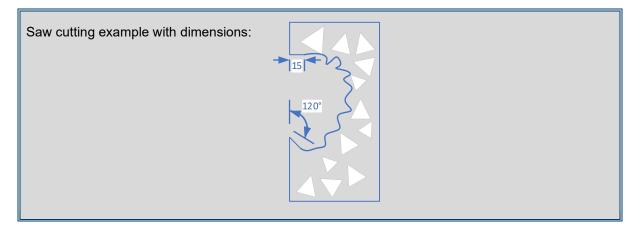
The area of repair shall be delineated to form square to rectangular shapes.
