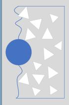
Where steel is fully exposed, the concrete behind the bar may need to be removed to create better embedment. This is also necessary in cases where the steel is corroded so the whole bar can be cleaned.
