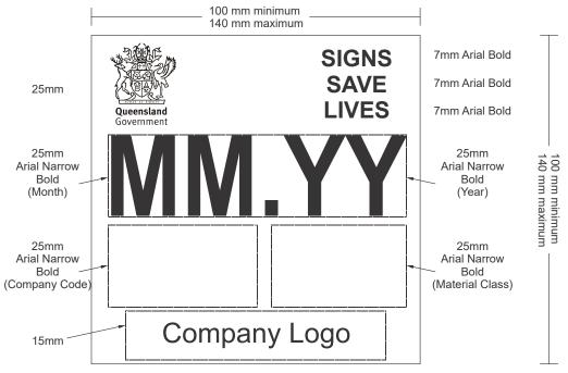
The markings detailed in above shall be black. The lettering in (b), (c) and (d) shall be 25 mm high and located so as to be visible after the sign is erected and not in a position likely to be obscured by stiffener rails or mounting posts. The legend described in (e) shall be located next to the corporate logo in a clear location and shall not exceed the height of the logo.
